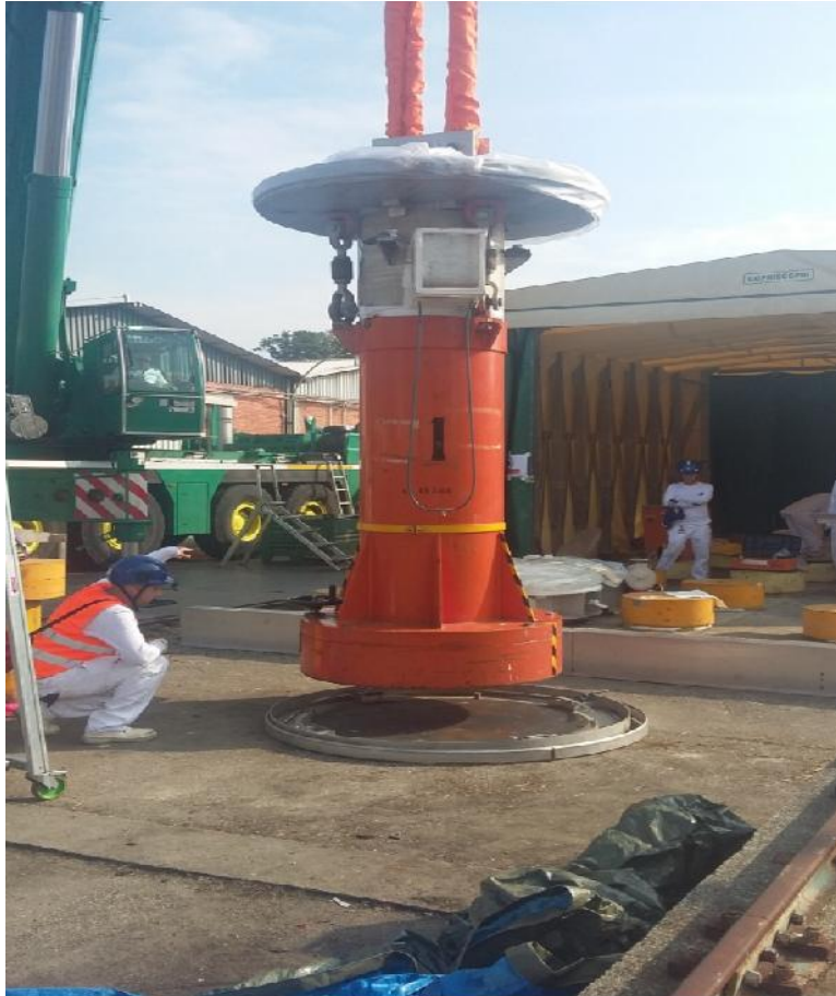
Figure 3: Cold test for the transfer of spent fuel pots from dry-well pits to the dry storage in ESSOR reactor hot cell
