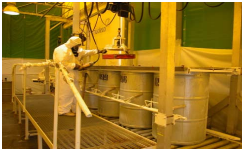
Itrec - Overpack preparation
