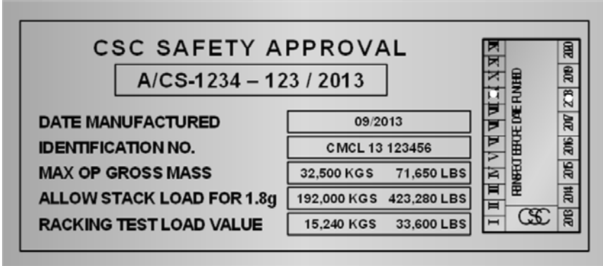
Figure 4.2 CSC safety approval plate with next examination date
