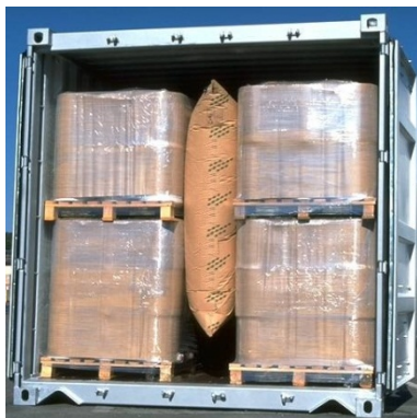
Figure 7.9 Gap filled with a central dunnage bag
