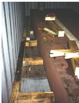
Figure 7.45 Transverse blocking of steel slab
