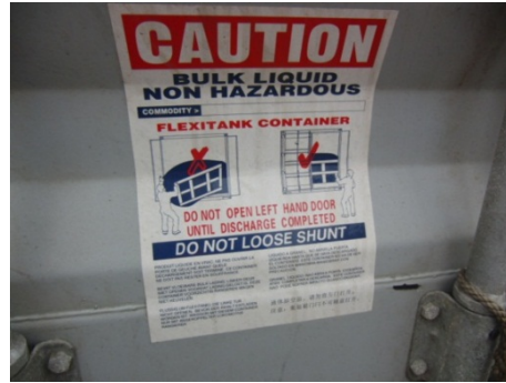
Figure 7.52 Flexitank warning label
