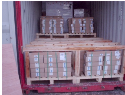
Figure 7.2 Timber temporary floor
