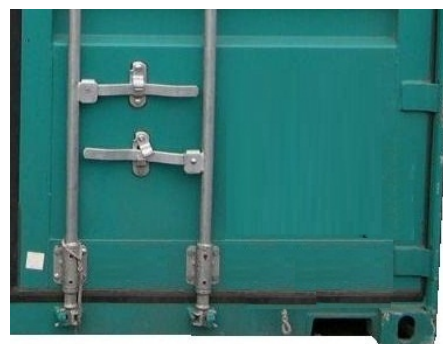
Figure 5.27 Handles between bars
