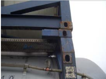
Figure 4.9 Step back with secondary side lift aperture
