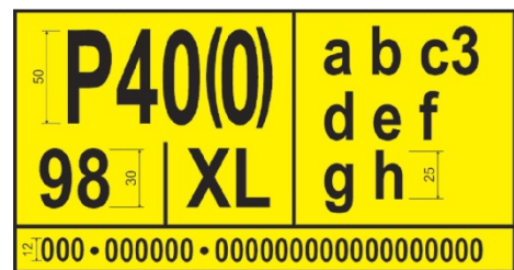
Figure 4.5 Yellow operational mark for trailers
