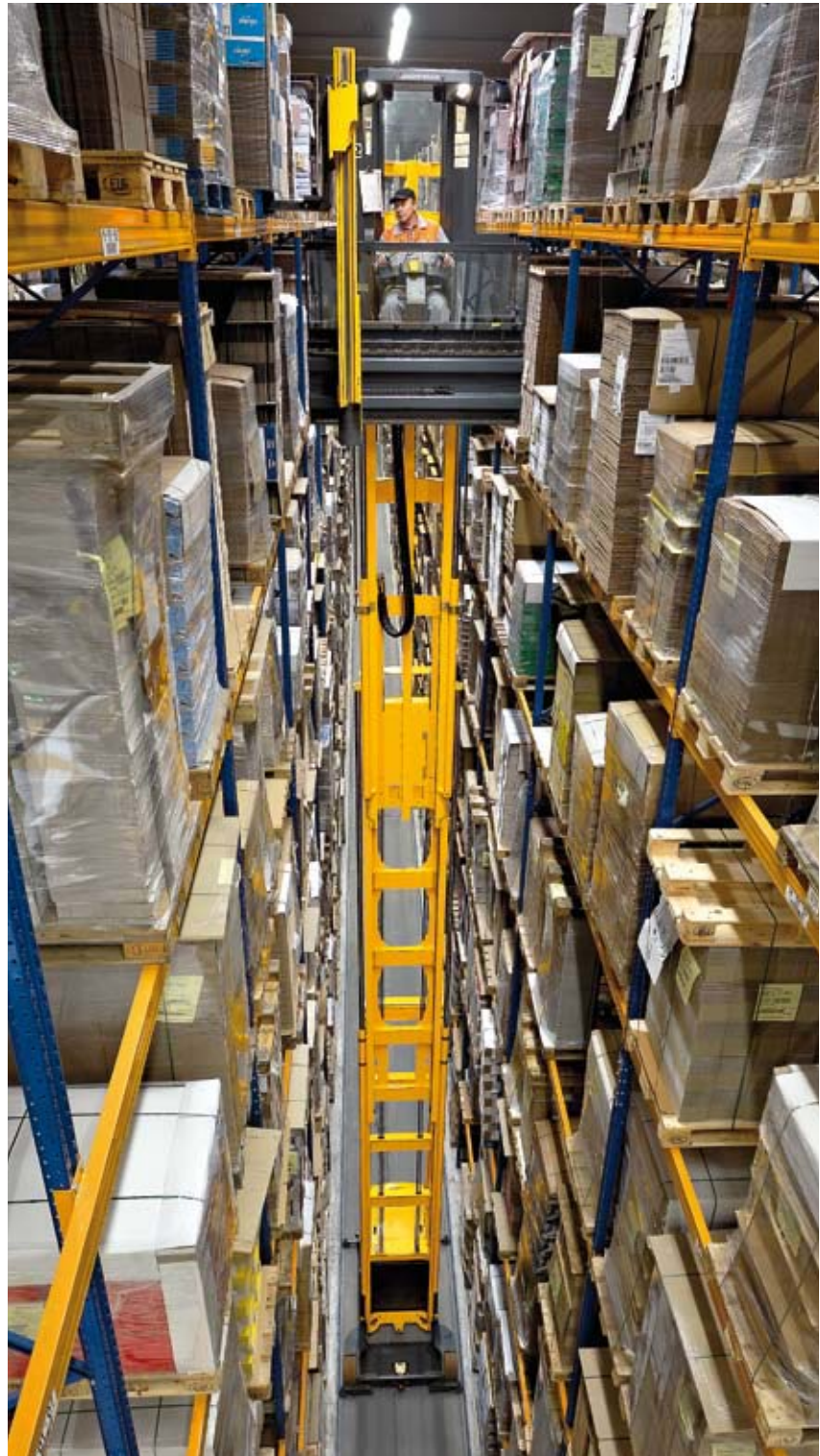
EKX 515, lifting height 16.5 m
