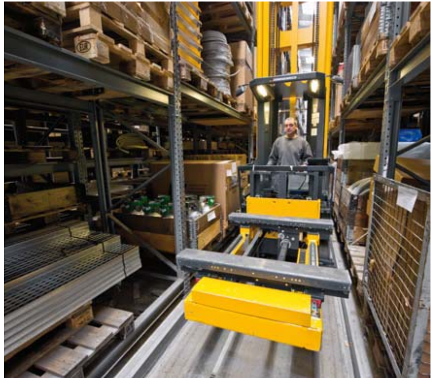
EKV 515, hydraulically adjustable telescopic fork
