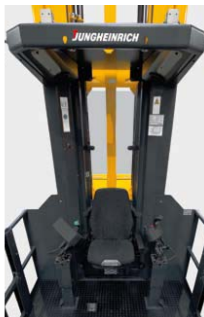
EKK 515, split operator consoles and conversion to a picking truck
