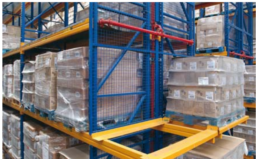
P&D location with projecting bearing surfaces
