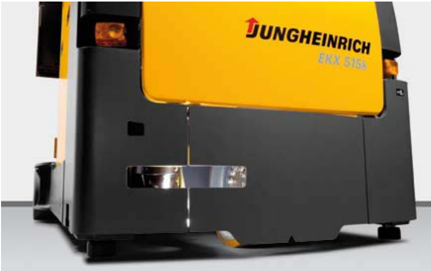
Protected laser scanner in an EKK 515k
