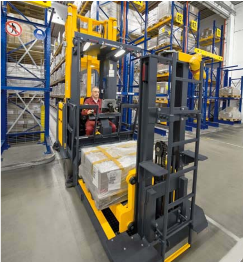
EKK 513, telescopic fork with auxiliary lift in front of the fork and emergency escape ladder
