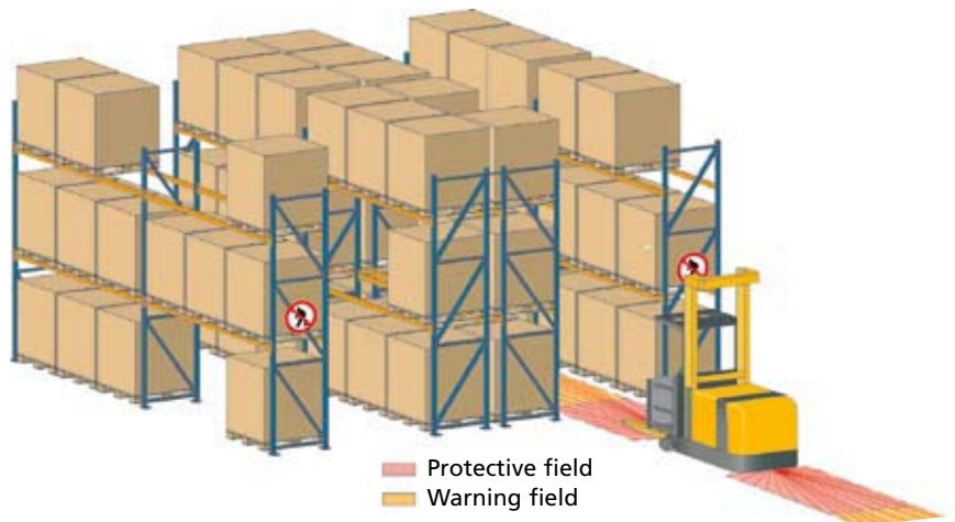
Monitoring fields of the mobile PSS
