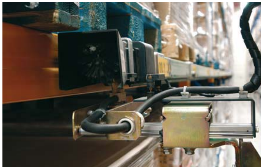
Enclosed conductor rail with current collector
