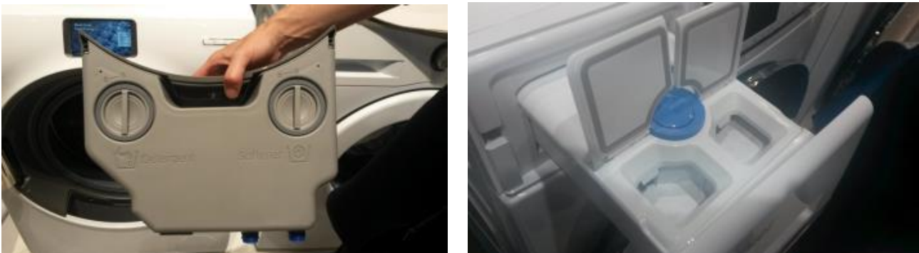
Figure 4.8: Automatic dosage system presented at the IFA 2015 fair in Berlin by Samsung (top) and Haier (below); (source: own pictures)
