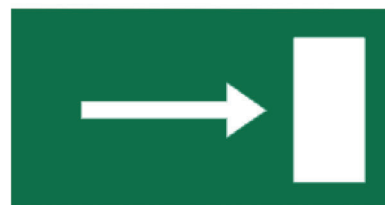
DIRECTION OF EMERGENCY EXIT
