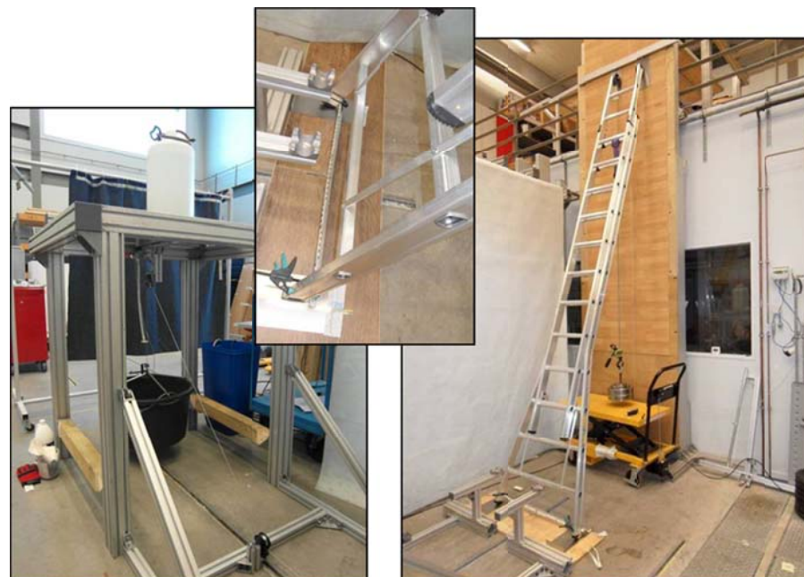
Figure 1 - Impression of the base slip test site. Right, the vertical test wall with one of the samples on stainless steel. Left, the contraption that guides a thin steel wire along pulley's to transfer the weight of a bucket filled with water horizontally onto the lowest step of the ladder. In de middle a top view at the feet standing on stainless steel.
