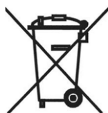
Figure 6: Symbol for the marking of EEE according to Annex IX of the WEEE Directive
