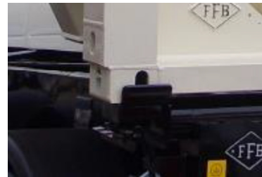
Figure 10-88 Backstop (viewed from rear of trailer)
