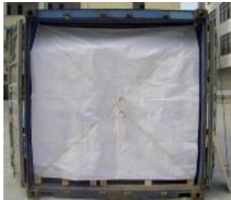
Figure 10-42 Tarpaulin used solely to prevent small and light packages from falling out when stowed close to the door.
