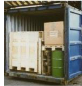
Figure 10-40 Mixed stow, use of pallets
