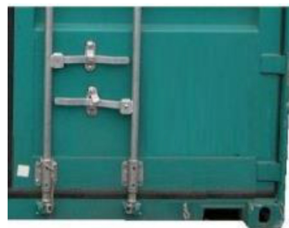
Figure 6-19 Handles between bars
