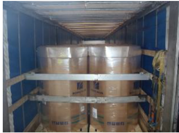
Figure 10-15 Blocking cross beams with limited strength due to physical connection
