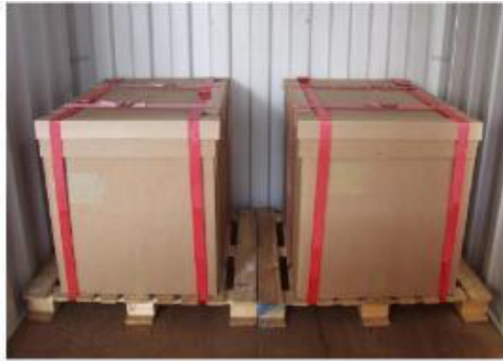
Figure 10-11 Cargo firmly secured to pallets by textile lashings
