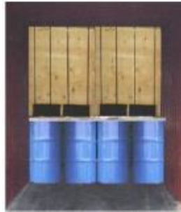
Figure 10-39 Mixed stow, dry over wet goods
