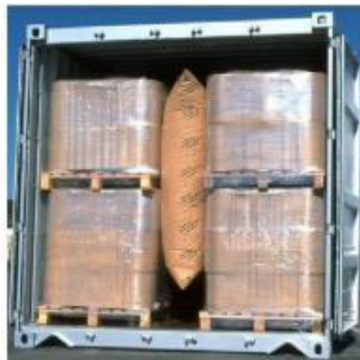
Figure 10-12 Gap filled with a central dunnage bag
