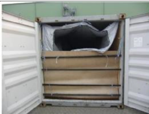
Figure 10-79 CTU with liner bag for accommodating a sensitive bulk cargo
