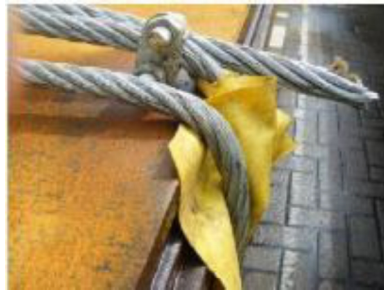
Figure 10-17 Poor edge protection
