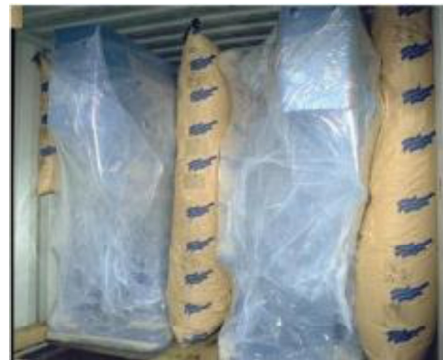
Figure 10-13 Irregular shaped packages blocked with dunnage bags
