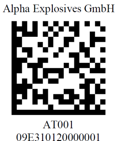
Figure 34: Example of Data Matrix code for identifying and tracing explosives
