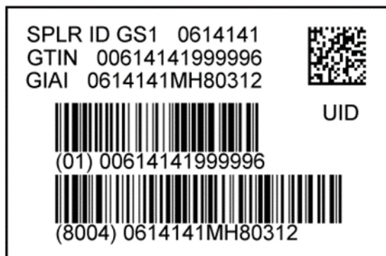
Figure 40: Example of a label item marking according to DoD IUID Equivalents
