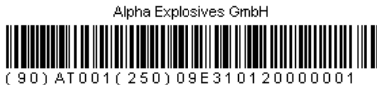
Figure 33: Example of barcode for identifying and tracing explosives
