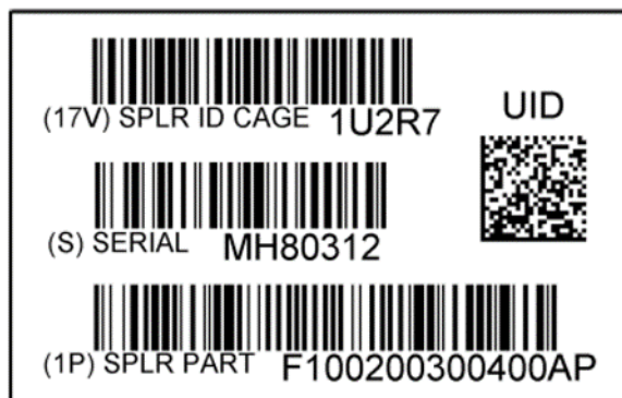
Figure 39: Example of a label for item marking according to DoD Construct #2
