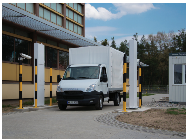
EUSECTRA outdoor lab with portal monitors which simulates border controls.
