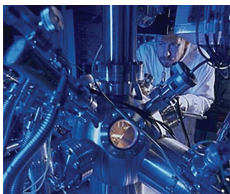
Photoemission spectrometer to study surface phenomena relevant for spent fuel corrosion processes.
