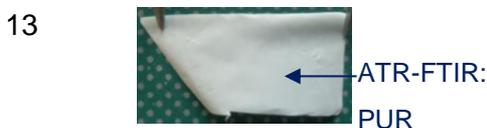
The Al foil on the bottom of part A is completely dissolved. → ATR-FTIR: part A (bottom, Al foil removed) = polyester urethane (adhesive)
