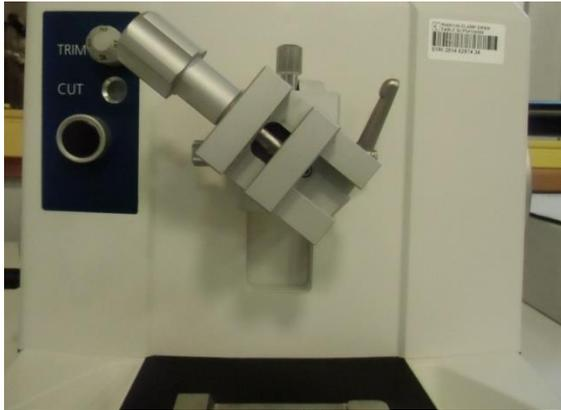
Reassemble the remaining parts of the standard object clamp.
