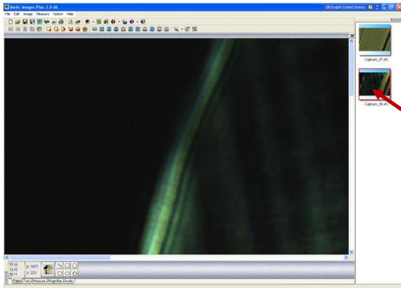
Go to the window "Motic Images Plus 2.0 ML" and load an image. You can either select one of the photos taken before from the right side of the window or load an image from a file. IN the latter case, open the menu "File" and select "Open".
