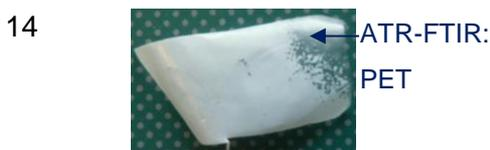
To confirm that the "white layer" on the bottom side of part A is a reverse printing and to check what is below, try to rub it off with a paper towel soaked in ethyl acetate (requires some force!). → PUR adhesive and the printing are removed. → ATR-FTIR: part A (bottom, print removed) = PET → same like outside → PET-monolayer
