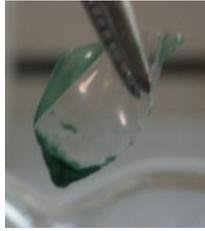
Check whether **part A** consists only of PA by dissolving it completely in cold HCOOH:
