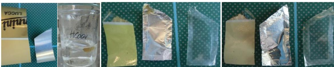
Figure 4 Sample (PET/print/<sup>PUR</sup>Al foil/<sup>PUR</sup>PE) before and after boiling in HCOOH for 5 min. Resulting 3 separated layers: PET/print, Al foil, PE (top and bottom view shown)
