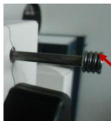
Pull out the metal bar in the upper part of the microscope. Now the live picture of the camera (Moticam 10) can be seen on the screen (in the "Motic Live Imaging Module" window).
