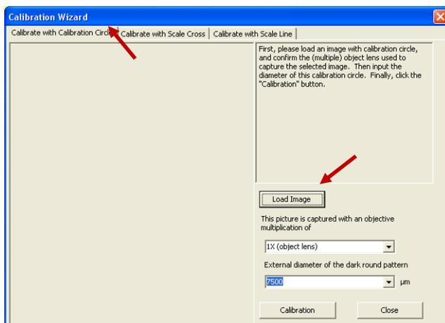
The window "Calibration Wizard" will open. Go to tab "Calibrate with calibration circle" and click the button "Load Image".
