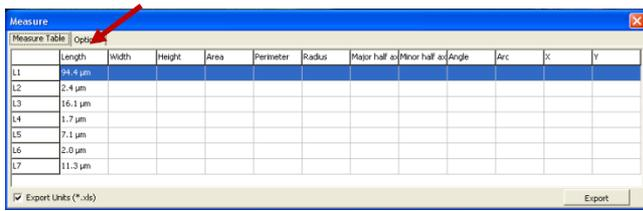
A new window ("Measure") opens. The tab "Measure Tables" shows the length of each drawn line.
