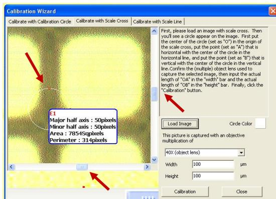
The selected photo will be opened in the "Calibration Wizard" window. Use the scroll bars on the right and on the bottom to move to the centre of the photo. There you will find a white circle with two red dots and a dialog box that shows the current dimension of the white circle.
