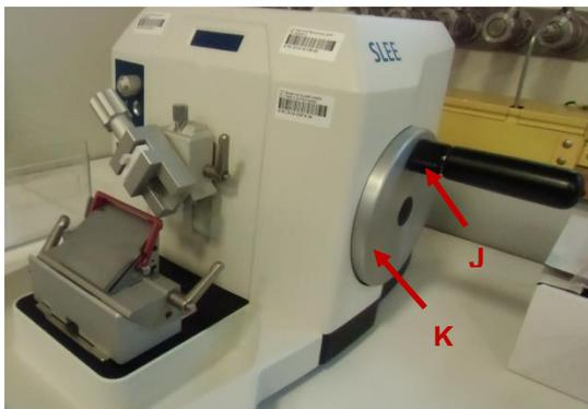
Before trimming, check again the position of the blade holder. Loosen the hand wheel stop **(J)** on the right and slowly turn the hand wheel **(K)** on the right to move the specimen holder down.
