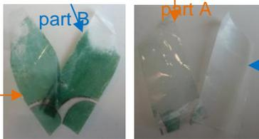
Remove the printing from the bottom of **part A** and from the top of **part B** to check what is below:
