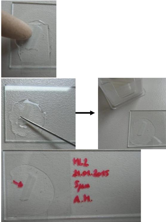
Apply some more mounting medium on top of the sectioning tape and cover everything with a cover slip. Again gently press with the wooden shaft of the paint brush to remove eventually present air bubbles. Clean the dissecting needle with a paper towel.
