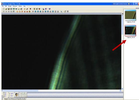
Readjust the focus again if necessary and adjust the position of the microscope slide to see all the layers of the sample in the live picture on the screen. Go to the tab "Video Capture" (see camera symbol) and click "Capture" to take a snap shot of the current camera view.
