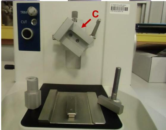
Install the corpus of the standard object clamp **(C)** at the object orientation. Use an Allen key (size 3 x 100 mm) to fasten the two screws.
