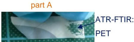
**Go back to step 2** – To confirm that the “white layer” on the bottom side of **part A** is a reverse printing and to check what is below, try to rub it off with a paper towel soaked in **ethyl acetate** (requires some force!). → PUR adhesive and the printing are removed. → ATR-FTIR: **part A** (bottom, print removed) = **PET** → same like outside → PET-monolayer
