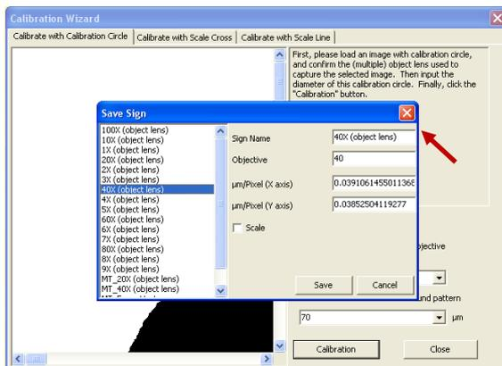
A new window "Save Sign" will open. Select a "Sign Name" from the column on the left (e.g. "40X (object lens)") or define a new one. Then click the button "Save".
