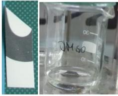
Cut a piece of the sample (complete laminate) (approx. 1 cm x 3 cm) and boil it for 1-2 min in DMSO to partly dissolve/swell the PE layer.
