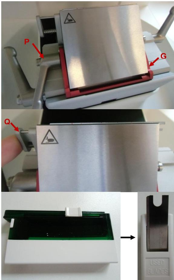
For changing the blade, refer to the user manual (see **Error! Reference source not found.**, chapter 7.5, p. 17). Fold down the finger protection guard (**G**) and loosen the metal arm on the left (**P**).
