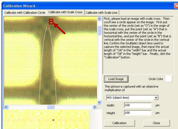
Move the cursor to the upper red dot (**B**). The cursor will transform into a hand. Now click on the red dot (**B**), drag it along the y-axis of the scale cross and drop it exactly at a certain scale division/bar (e.g. 5 bars = 0.05 mm = 50 μm away from the origin). The circle will deform into an ellipse.
