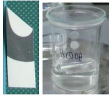
Cut a piece of the sample (**complete laminate**) (approx. 1 cm x 3 cm) and boil it for 1 min in **conc. HCOOH** to partly dissolve the adhesives above and below the aluminium foil.
