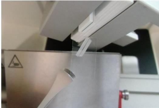
The moment the blade cuts off the section of the specimen, tear off the sectioning tape with the tweezers in your left hand. To obtain a good section, the cutting has to be performed at a continuous, average speed – neither too fast, nor too slow. It will need some training to find an optimum cutting speed and to coordinate all steps.
