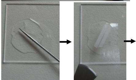
Spread the mounting medium and put the section tape on it. The sticky surface of the tape should face the microscope slide. Gently press with the wooden shaft of the paint brush to remove eventually present air bubbles.
