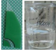
Cut a piece of the sample (**complete sample**) (approx. 1 cm x 3 cm) and boil it for 15 min in **HCOOH** to completely dissolve the PA layer on top of the sample
