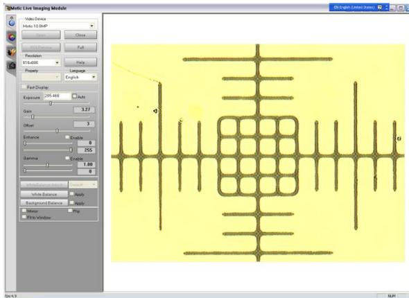
Readjust the focus again if necessary and adjust the position of the microscope slide to see the entire calibration circle or the origin of the scale cross. The calibration circle or the origin of the scale cross, respectively, should be in the centre of the picture. To properly align the scale cross, it may be necessary to slightly turn the camera.
