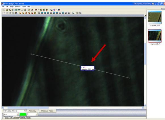
You can draw a line now. To do so, click and hold the left mouse button while dragging the line. The length of the line will be shown immediately in a small text box.
