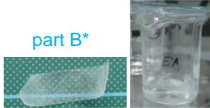
Separate polymer 2 and the PE layer:
