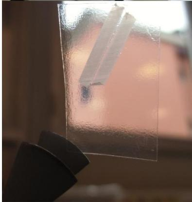
The section is acceptable from a first glance when the white strips cut off from the sandwich plastic plate are straight, homogeneous and eventual knife marks (periodic waves) are only barely visible. Whether the section is really fine, can only be seen afterwards during the microscopy.
