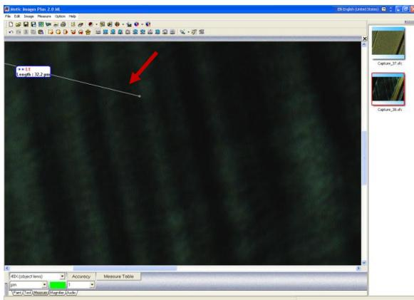
Start and end point of the line can be readjusted. Simply click on the start or end point with the left mouse button and drag and drop the point. Like this you can also elongate a line if the measurement area is bigger than the actual area shown on the screen.
