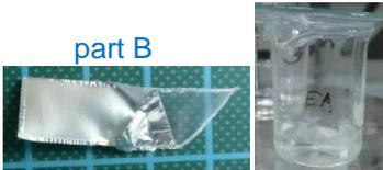
Separate polymer 2 and the PE layer:
