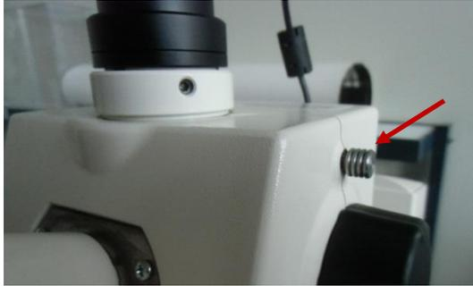
Push back in the metal bar to be able to view the sample in the eyepiece of the microscope.
