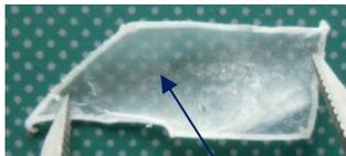
Remove the PUR adhesive on top of part B to check what is below:
