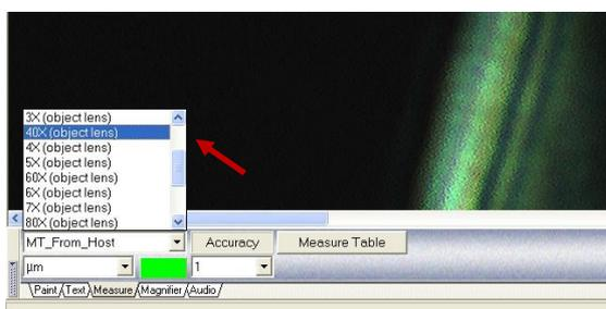
Select the correct object lens that was used to take the image. Open the tab "Measure" on the lower left of the window and select an object lens from the drop-down menu.
