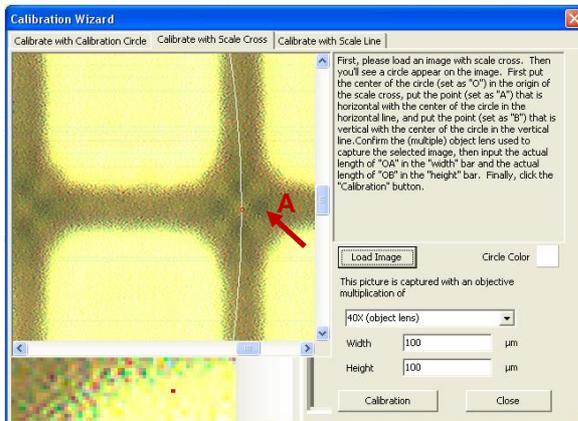
Then move the cursor to the right red dot (**A**). Again the cursor will transform into a hand. Click on the red dot (**A**), drag it along the x-axis of the scale cross and drop it exactly at a certain scale division/bar. Use the same distance as before at the y-axis (e.g. 5 bars = 0.05 mm = 50 μm away from the origin).
