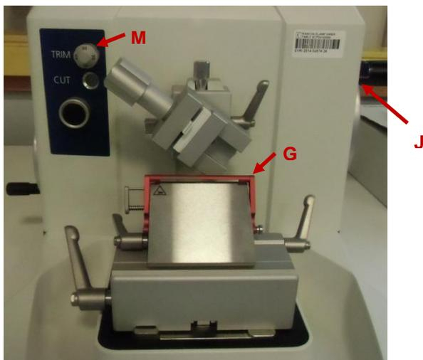
To start trimming, fold down the finger protection guard (red metal bar) **(G)**, loosen the hand wheel stop **(J)** and slowly turn the hand wheel **(K)** on the right clockwise while pressing the grey "TRIM" knob **(M)** on the left. With every turn of the hand wheel, the specimen holder will move 30  $\mu\text{m}$  towards you as set before on the "TRIM" knob **(M)**.
