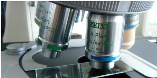
Adjust the focus so that the sample is clearly visible. For sufficient magnification use the 40x object lens.
