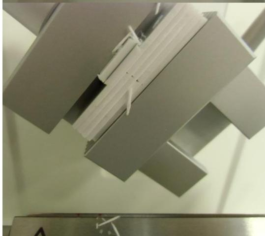
After some turns of the hand wheel **(K)**, the specimen will touch the blade and sections of 30  $\mu\text{m}$  thickness will be cut from the specimen. Continue like this until a plane and clear specimen surface is obtained (incl. the white plastic plates in between which the specimen is sandwiched). Do not perform the trimming sections too fast to avoid damage of the specimen surface.
