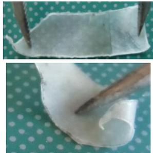
Having a closer look to the edges of part B after treatment with  $H_2SO_4$ , you can see that there is no black line visible. → There is no EVOH layer sandwiched between two PE layers. → The PE layer is probably a monolayer.
