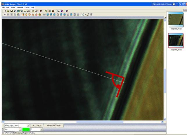
The measurement should be carried out perpendicular to the layers.
