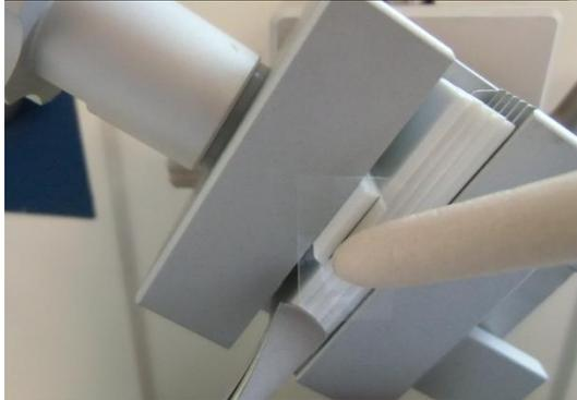
Remove the paper from the backside of the sectioning tape and stick the sectioning tape to the surface of the specimen. Carefully press it to the specimen surface, e.g. with the wooden backside of the paint brush. Do not touch the tape with your fingers, use tweezers instead.
