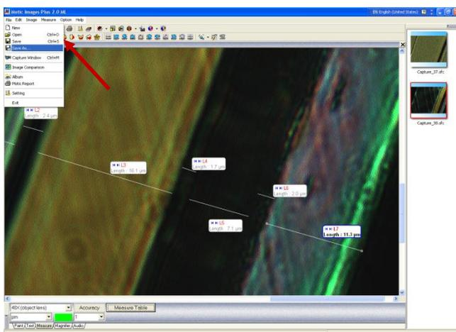
When you are finished, save the file. To do so, open the drop-down menu "File" in the upper left corner of the screen and select "Save As".
