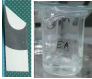
Cut a piece of the sample (complete laminate) (approx. 1 cm x 3 cm) and boil it for 1 min in **ethyl acetate** to partly dissolve/swell the adhesives on top of and below the aluminium foil.
