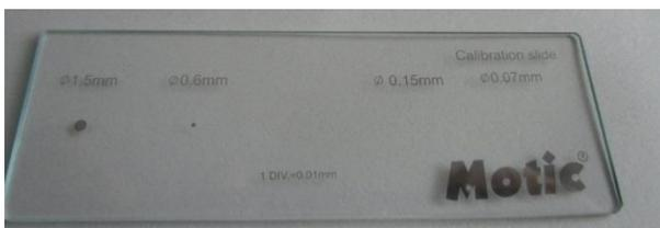
Take the microscope slide with calibration circles and scale cross and place it on the specimen holder.
