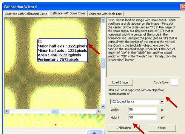
If you positioned each of the red dots (**A**, **B**) with the same distance to the origin of the scale cross, the pixel number for the x- and y-dimension ("Major/Minor half axis") of the circle must be the same. If not, readjust the positions of the red dots. Sometimes it can be necessary to reposition/re-centre the entire circle.
