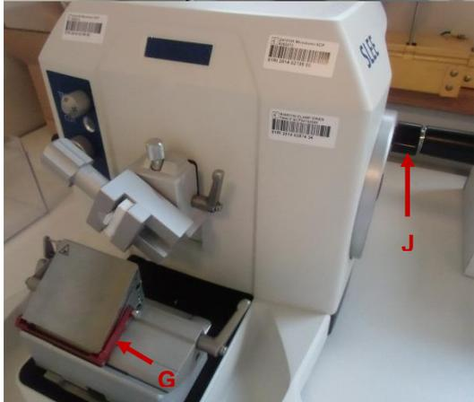
To prepare the microtome section, fold down the finger protection guard (**G**) and loosen the hand wheel stop (**J**).
