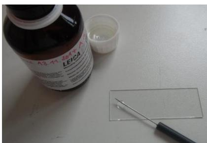
If an acceptable section was obtained, take a microscope slide and apply some mounting medium with the dissecting needle.
