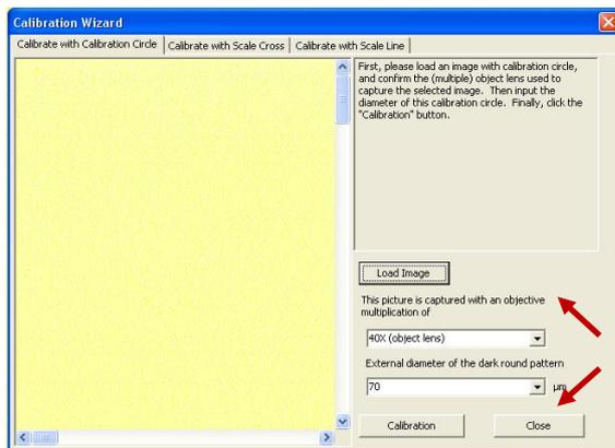
Enter the diameter [ $\mu\text{m}$ ] of the selected calibration circle and specify the object lens (e.g. 10x, 20x or 40x) with which the snap shot was taken. Then click the button "Calibration" and the calibration is done automatically.
