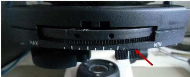
Use the sliding knob to set the aperture diaphragm to approx. 2/3 or 4/5 of the diameter of the objective exit pupils as described in the instrument manual 0. Insert the eyepiece in the tube again when ready.
