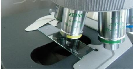
Swing in the 10x object lens and adjust the focus so that the object is clearly visible.
