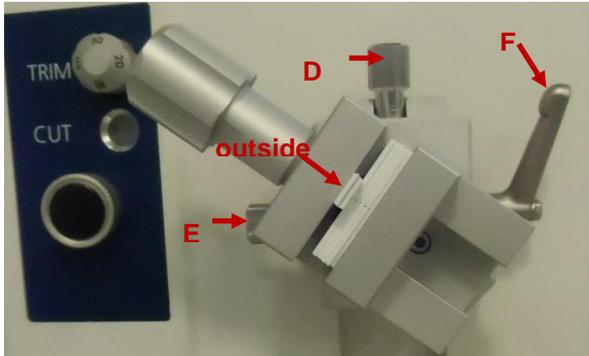
Insert the folded plastic plate into the standard object clamp. Again the non-food contact side (outside) of the sample should face upwards.
