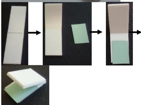
Insert the sample strip in between one of the foldable plastic plates. Pay attention whether the non-food contact side (outside) of the sample faces upwards or downwards. To avoid confusion, it should always face upwards.
