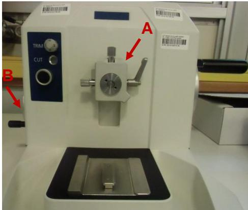
The microtome should be equipped with the object orientation **(A)**. If not, install it and fasten all 4 screws using an Allen key (size 4 x 150 mm).
