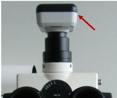
NOTE: Do not change the position of the camera after having taken the snap shot for calibration. Otherwise a new snap shot should be taken to carry out the calibration.
