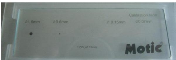
Place a high-contrast specimen on the specimen holder (e.g. the calibration slide → circle with 0.15 mm diameter).
