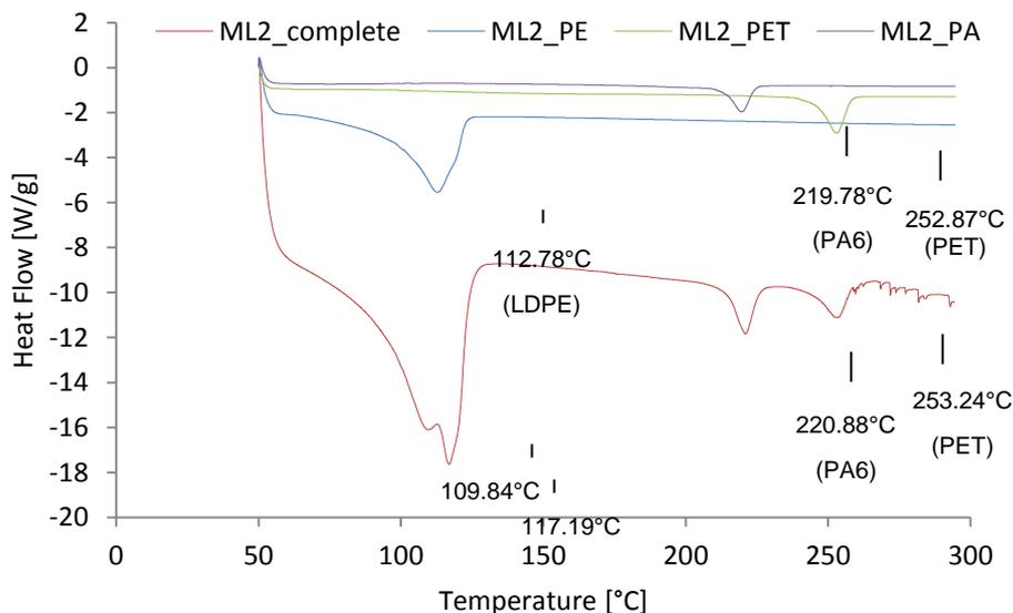
Figure 8 DSC diagrams of a laminate (PET/acrylate printing//<sup>PUR</sup>Al foil//<sup>PUR</sup>PA//<sup>PUR</sup>PE) and its single polymer layers (PET, PA, PE) after separation
