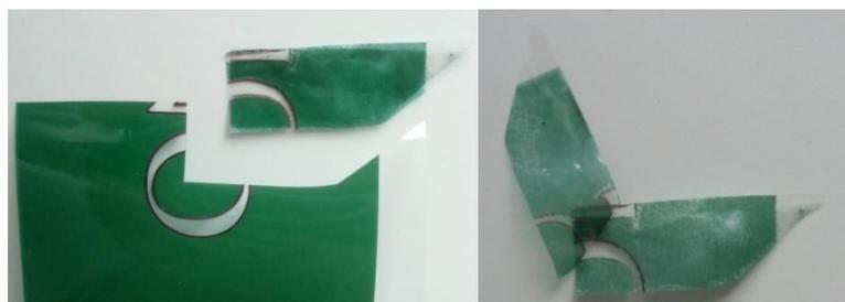
Figure 1 Laminate with reverse printing (PA/print/<sup>PUR</sup>PE) after boiling in ethyl acetate for 2 min
