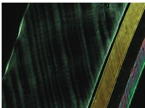
The field of view will appear dark now because the polarisers are crossed. Only birefringent (i.e. anisotropic) objects (e.g. polymer films where polymer chains have an orientation, e.g. due to shear stress in the die or due to stretching during extrusion) will display a colour now (white or brightly coloured) (see 0, 0).
