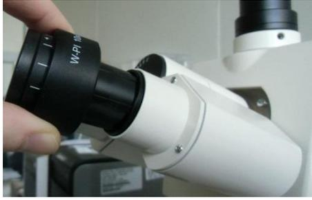
To set the aperture diaphragm (contrast), remove one eyepiece from the tube (it can be pulled out) and look into the tube with your naked eye.
