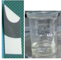
Cut a piece of the sample (**complete laminate**) (approx. 1 cm x 3 cm) and boil it in **conc. HCl** to partly dissolve the aluminium foil
