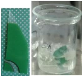
Now that you know, that the sample is reverse printed, you should check that you did not dissolved anything else during step 1 apart from the PA layer. Therefore, try to separate the PA layer from the **complete sample** and check its bottom side:
