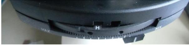
Switch the turret disk of the condenser to position "H" for brightfield.
