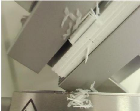
Then perform another 5-10 sections of 5  $\mu\text{m}$  without pressing the "TRIM" knob **(M)** to really obtain a smooth specimen surface. When finished, fasten the hand wheel stop **(J)**.
