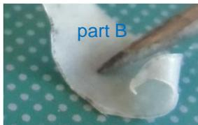
Check whether **part B** is really a monolayer or whether it consists of coextruded layers, e.g. two PE layers with an EVOH layer in between:
