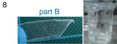
Separate the PA and PE layer of part B:
