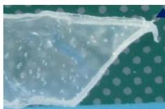
Separate the PA and PE layer of part B:
