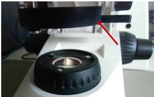
To view the object in plane polarised light, swing the polariser in the beam path.
