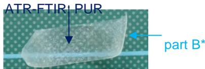
immerse **part B** again for 10 s in **boiling conc. HCl** → the aluminium layer is dissolved immediately → **part B\*** (adhesive/polymer 2/adhesive/PE) remains → ATR-FTIR: **part B\*** (top) = **polyester urethane (adhesive)**, **part B\*** (bottom) = **PE**
