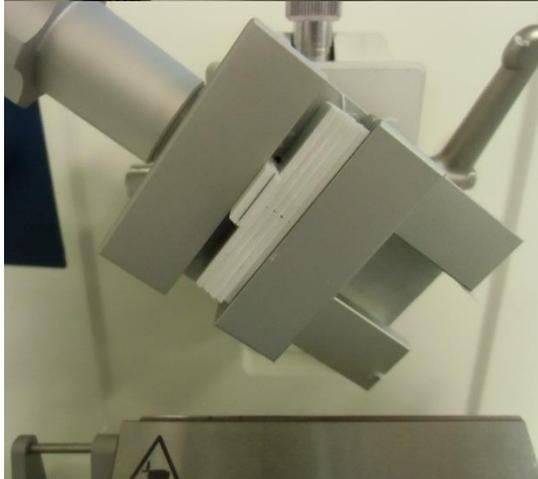
The blade and specimen block should be completely clean before you proceed with the next steps.
