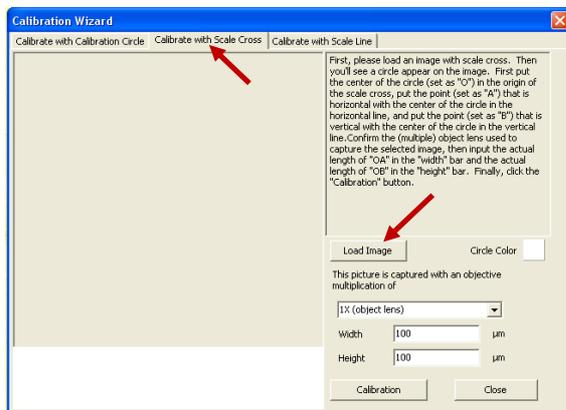
The window "Calibration Wizard" will open. Go to tab "Calibrate with scale cross" and click the button "Load Image".
