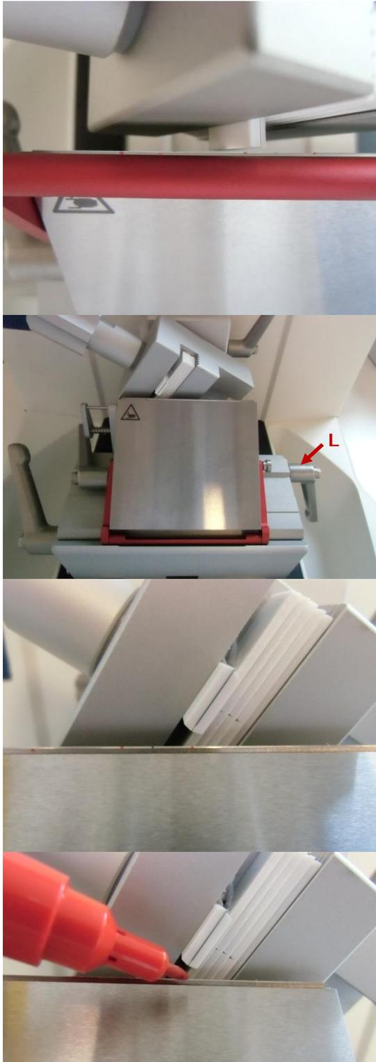
The blade holder should be positioned close to the specimen but the blade should not yet touch the specimen. 0.5-1 mm of distance between blade and specimen are enough. Otherwise trimming will take much longer. If necessary, reposition the blade holder by loosening the metal arm (**H**) on the lower left. (NOTE: Refasten the hand wheel stop (**J**) before you readjust the blade holder position.)
