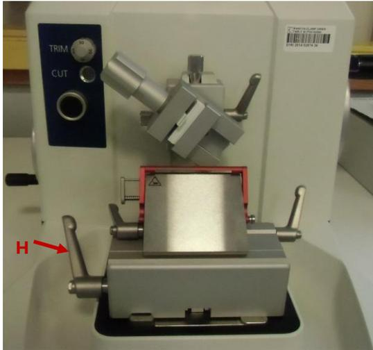
Put the blade holder on the metal rail and fasten it by pulling tight the metal arm **(H)** on the lower left.
