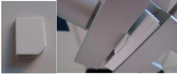
NOTE: If later on problems appear and the sections are not cut off completely from the specimen, the right edge (which will be the upper edge when inserted into the standard object clamp) of the foldable plate with the sample strip in between can be cut off with a razor blade.
