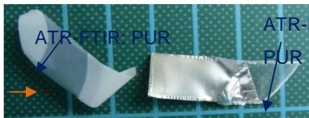
...and **part B** (adhesive/polymer 2/adhesive/PE) can be peeled off from the bottom of the aluminium foil.
