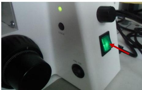
Switch on the microscope.
