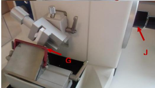
Fasten the hand wheel stop (**J**) and fold up the finger protection guard (**G**) after the section.
