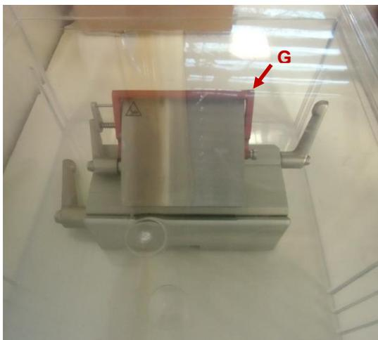
**After** having inserted the specimen and adjusted the object orientation, take out the blade holder from the plastic box. Be careful when handling the blade holder. The blade is very sharp and you can easily injure yourself when touching it. The red metal bar ("finger protection guard") (**G**) should always be folded up to shield the blade and to prevent accidentally touching it.
