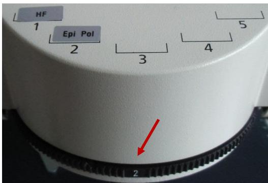
To view the object in crossed polarised light, swing in the analyser module (filter No. 2 "Epi Pol") on the reflector turret in addition.
