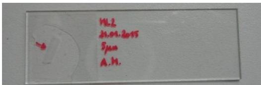
Take the microscope slide with the microtome section of the sample and place it on the specimen holder.
