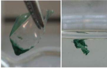
Part A is dissolved immediately. Only the green printing ink film remains in the beaker. → Part A seems to consist only of PA.
