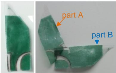
The PA layer (**part A**) can be peeled off. The printing sticks to both sides (the bottom of **part A** and the top of **part B**).
