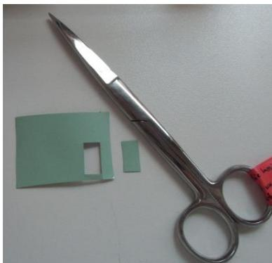
Cut a strip of approx. 0.8 cm x 1.5 cm, but no bigger than 1 cm x 2 cm, from the multilayer plastic film sample. Use the dissecting scissors to do so. With an ordinary pair of scissor, you might squeeze the edges of the sample strip.
