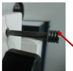
Pull out the metal bar in the upper part of the microscope. Now the live picture of the camera (Moticam 10) can be seen on the screen (in the "Motic Live Imaging Module" window).
