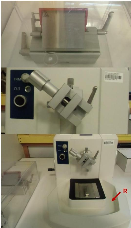
Clean the blade holder with a dry paint brush and put it back into the plastic box for storage. Be careful again not to injure yourself while handling the block.
