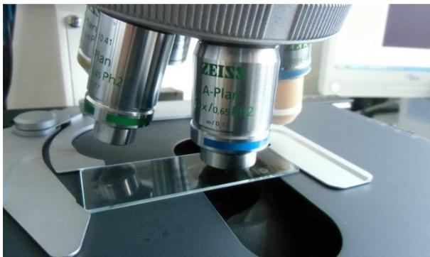
Select the object lens that needs to be calibrated and adjust the microscope focus to view the appropriate calibration circle or the scale cross (see Table 10).
