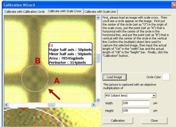
The circle must be positioned in the very centre (origin) of the scale cross. If necessary, reposition it. To do so, move the cursor above the white circle. The cursor will transform into a cross. Now click on the circle with the left mouse button and drag and drop it.
