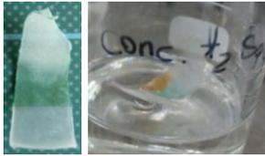
Check whether part B is really a monolayer or whether it consists of coextruded layers, e.g. two PE layers with an EVOH layer in between:
