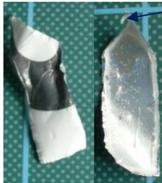
The edges of the PE layer are swollen and the adhesive that bonds polymer 2 to the aluminium foil is partly dissolved.
