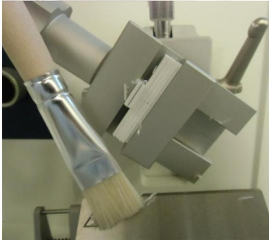
Remove section material from the blade and the specimen holder with a dry paint brush. Be careful not to cut yourself.
