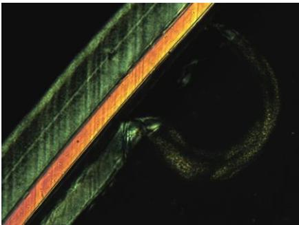
Carefully "scan" the entire microtome section from head to tail. It may happen that certain parts are damaged and one or more of the sample layers can be delaminated. Try to find an intact part of the section to continue. Otherwise you have to prepare a new section.
