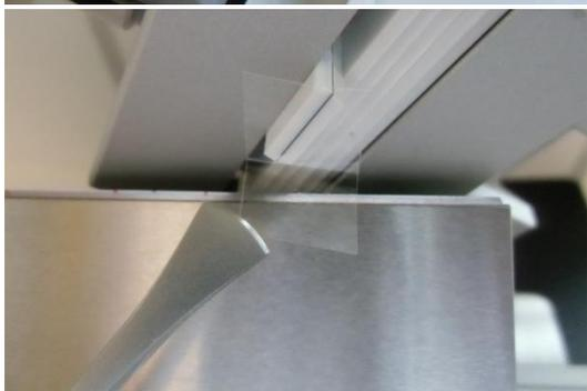
Turn clockwise the hand wheel (**K**) on the right with your right hand without stopping until the specimen completely passed the blade, while at the same time you keep holding the sectioning tape with some tweezers in your left hand.
