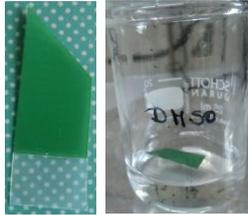
Cut a piece of the sample (**complete laminate**) (approx. 1 cm x 3 cm) and boil it in **DMSO** to swell the PE layer on the bottom of the sample.
