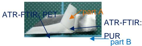
**after 30 s** the adhesive that laminates **part A** (PET/print) to the aluminium foil is (partly) dissolved, while the aluminium foil is only dissolved at its edges
