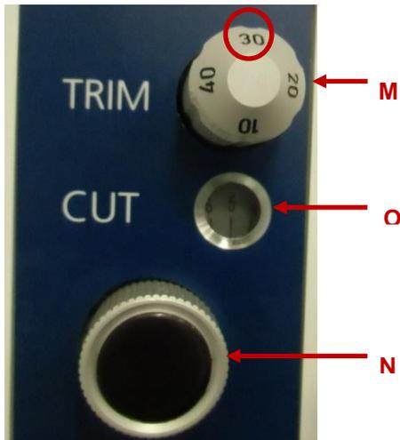
Set the trimming thickness at the upper grey knob **(M)** on the left front side of the microtome, labelled with "TRIM". It can be varied from 10 to 40  $\mu\text{m}$ . Usually a trimming thickness of 30  $\mu\text{m}$  is ok.
