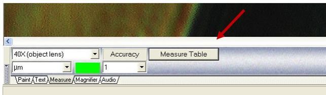
A table that lists the dimensions of all lines drawn can be accessed via the button "Measure Table" in the lower left corner of the screen, tab "Measure".
