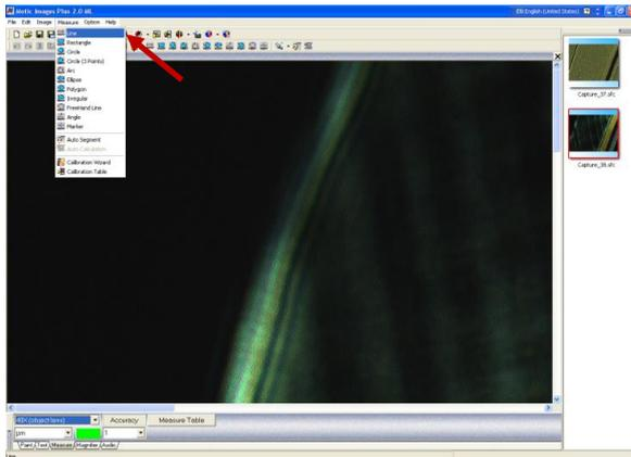
To measure the thickness of the layers in the picture, open the menu "Measure" on the upper left of the window and select "Line" from the drop-down menu.
