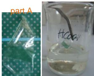
Check whether **part A** consists only of PA by dissolving it completely in cold HCOOH:
