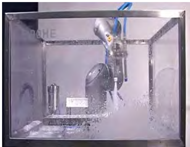
Figure 11. A washable robot can, nearly always, self wash using the basis of a CIP procedure.
