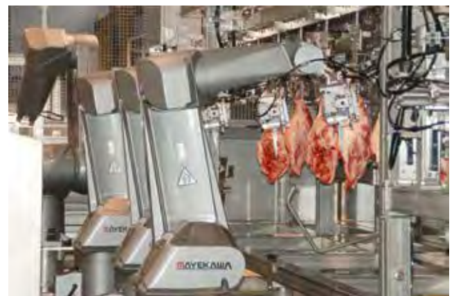
Figure 2. Fully automated ham deboning equipment integrating EHEDG guidelines.
