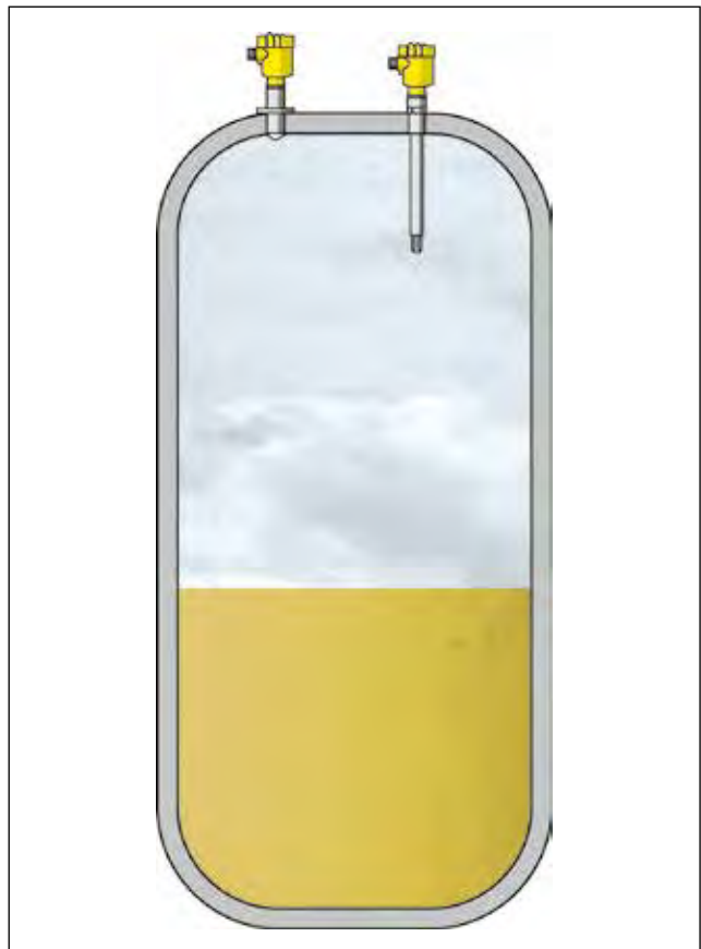
Figure 6. Non-contact level measurement with radar in storage tanks for liquid raw materials, intermediates and finished products.
