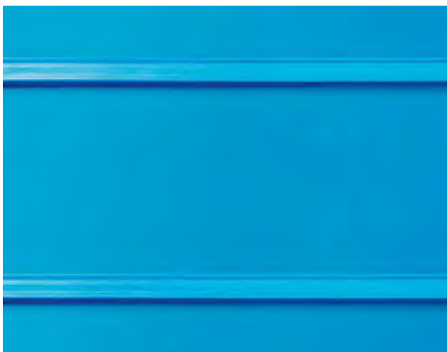
Figure 1. Underside of a traditional positive-drive conveyor belt with lateral teeth design.
