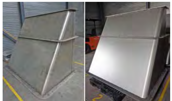
Figure 8. Large stainless steel container before and after treatment with the SUBLIMOTION-process.
