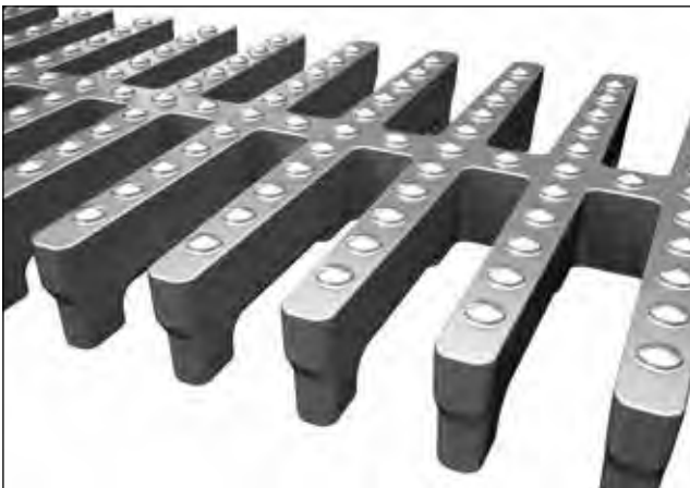
Figure 1. Gratings with open sides allow easy access of solid waste into the drainage system. The frame of some gratings holds back solid waste on the floor.
