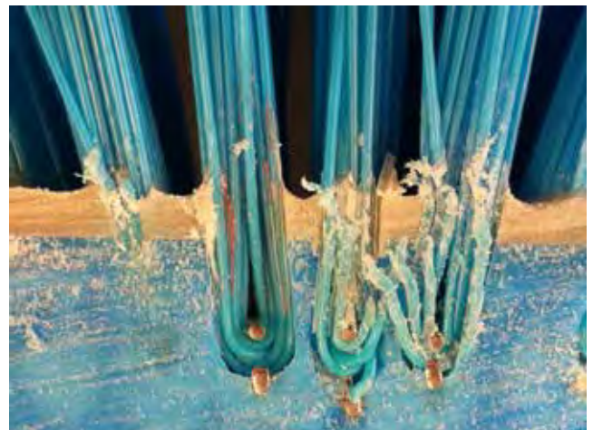
Figure 4. ‘Contamination’ (red) trapped between the bristles of a drilled and stapled resin set brush following decontamination using an industrial dishwasher. Channel depth is approximately 8 mm.
