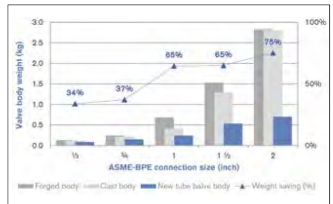
Figure 3. The tube valve body has a lighter thermal mass (up to 75 percent) than traditional forged or cast body alternatives and therefore saves energy.
