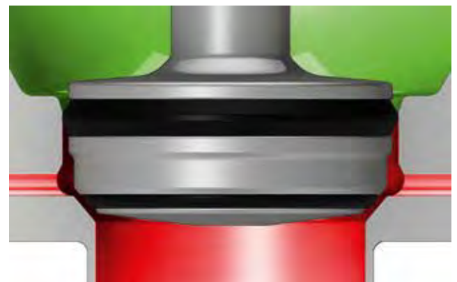
Figure 2b. Seat seal arrangement: radial top – axial bottom (open).
