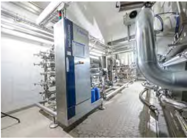
Figure 2. Impeccable hygiene is not only important for interior surfaces but for the system's exterior as well, including the tubular frame and stainless steel construction.
