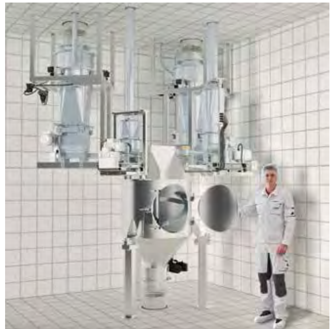
Figure 6. The amixon continuous mixer with four gravimetric dosing systems. The mixer rests on load cells. Filling and discharge nozzles are provided with flexible collars. The mixer's sealing valve is controlled so that the filling level in the mixer remains constant.
