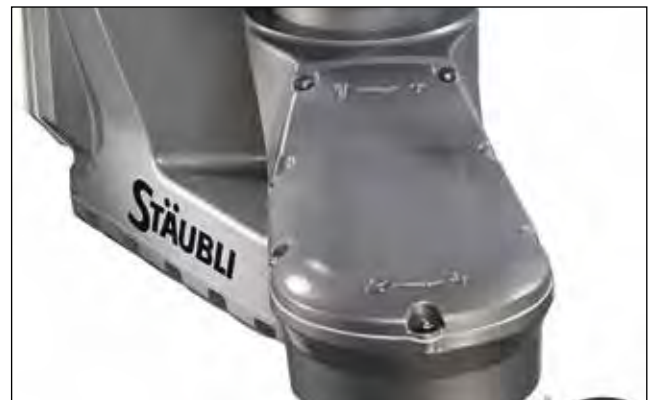
Figure 8. Protected robot against electrical exchanges by physical separation between stainless steel screws and aluminum based structure.
