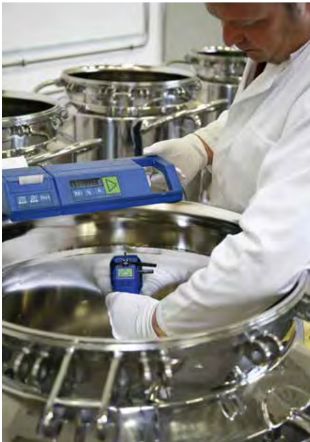
Figure 1. Surface roughness measurement in an electropolished stainless steel tank.
