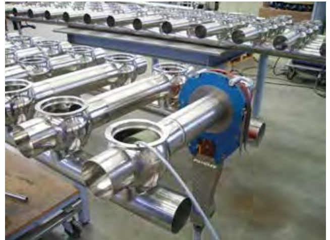
Figure 6. Orbital welding equipment on stainless steel tube with backing gas for the oxidation-free welds.
