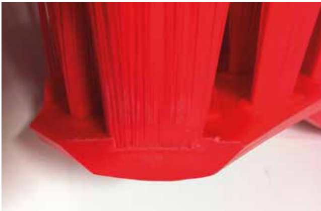
Figure 5a. Vertical cross-section through a UST brush to show its fully moulded construction.
