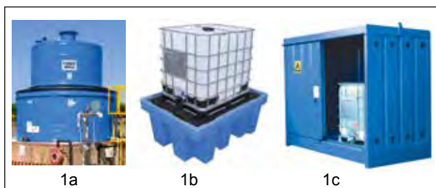
Figure 1. A range of external chemical storage devices, including bulk tanks (1a), IBC on a spillage container with a greater volume than the IBC (1b), and a smaller, leak-proof, external storage unit (1c).
