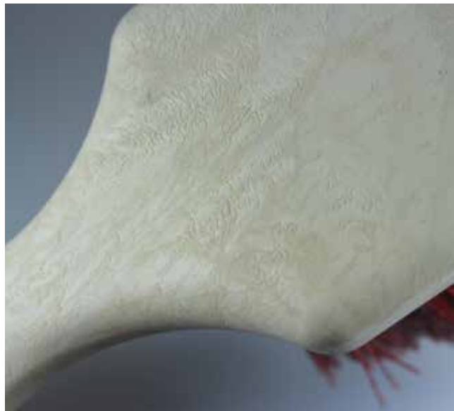
Figure 1a. Surface of a fused filament cleaning brush shows numerous creases that can provide harbourage for contamination.
