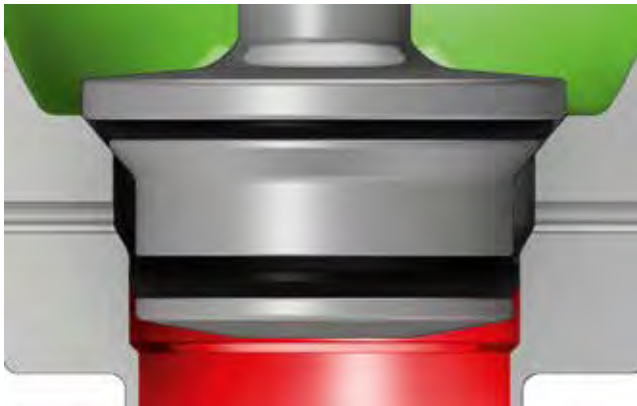
Figure 3a. Seat seal arrangement: axial top – radial bottom (closed).
