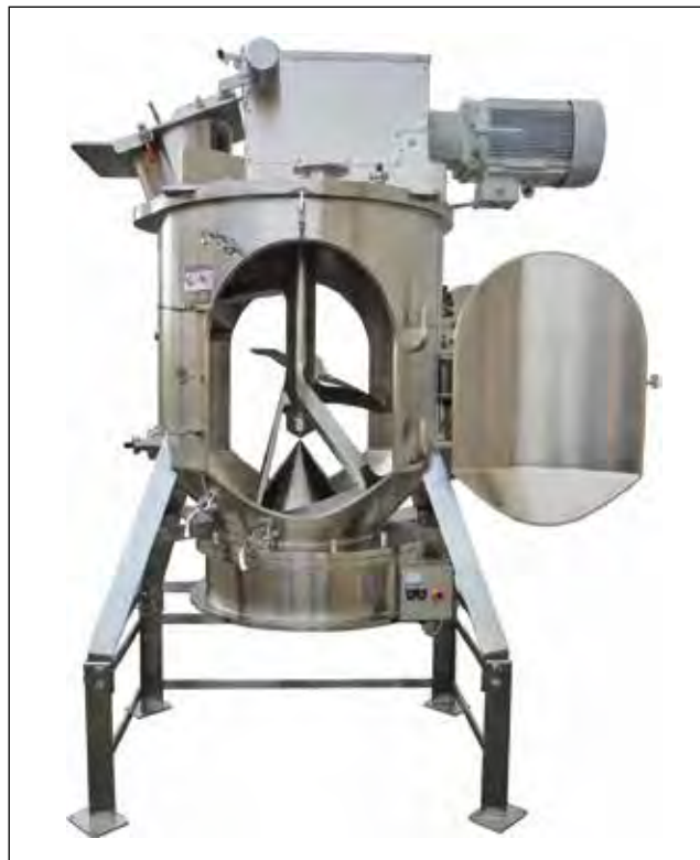
Figure 5. KoneSlid mixer with two large inspection doors.
