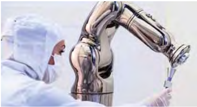
Figure 1. Probe head of a particle counter installed under a tribological element to detect emitted particles in an ISO1 environment according to ISO 14644-1.
