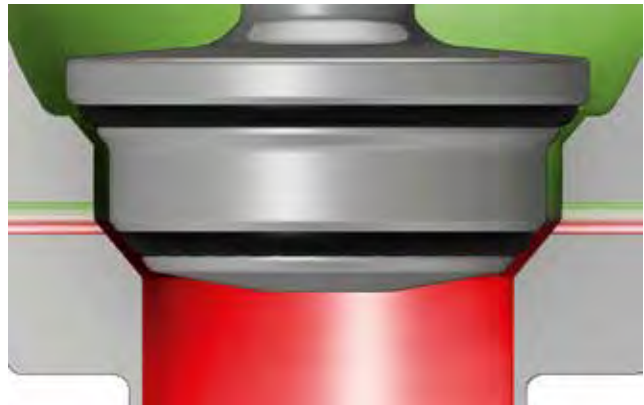
Figure 4b. Seat seal arrangement: axial top – axial bottom (open).
