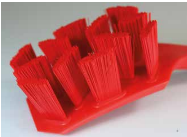
Figure 5b. The unique bristle pattern for the UST hand scrub brush, along with the fully moulded construction, minimises the possible risk of trapped contamination in accordance with EHEDG hygienic design principles.
