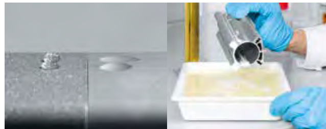
Figure 4a/b. (a) Surface with hydrophobic coating (left) compared to a surface with hydrophilic properties (right); (b) chemical testing of easy-to-clean coating on a cylinder barrel.
