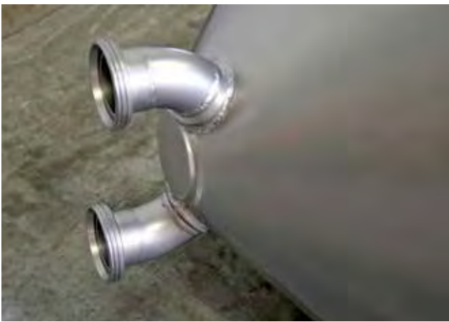
Figure 6. The same stainless steel component as shown in Figure 1, but now after treatment with the SUBLIMOTION-process. All contamination or impurities resulting from the fabrication are removed and at the same time the surface topography is reconditioned.
