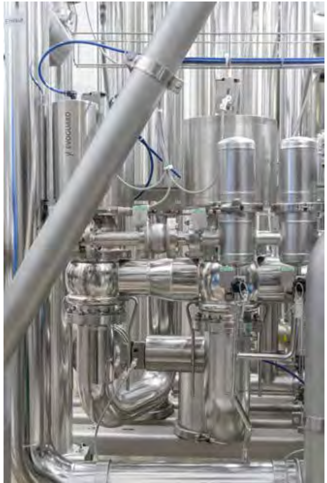
Figure 3. The use of leak-proof valve technology, especially double-seal valves, that are manufactured in-house guarantees immixture-free separation of the media involved.
