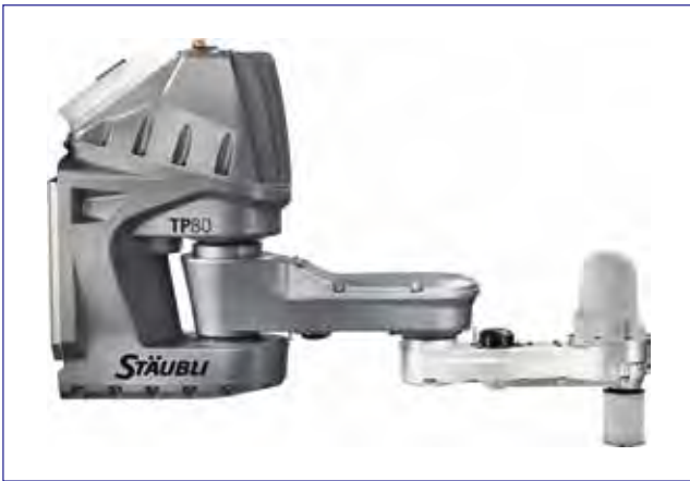
Figure 12. Fastest picking or decorating robot based on EHEDG recommendations, eliminating fixing screws in front of the product to produce smooth, sloped and opened surfaces.
