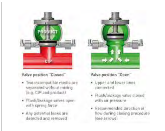
Figure 5. (Left ) Mix-proof separation of two media. (Right) Upper line and lower line connected.
