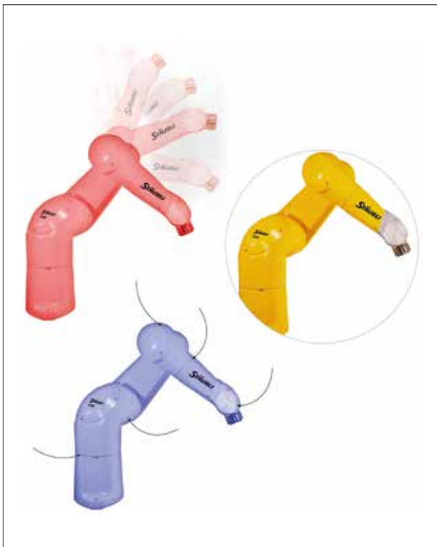
Figure 3. As the robot operates, it heats up to 60 to 70°C. When reducing its speed, or when static, it cools down quickly, producing condensation, and drawing the environment (air, humidity and bacteria) into the robot.
