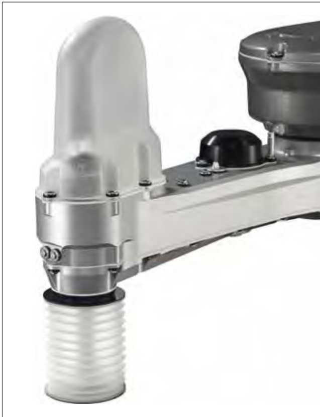
Figure 9. Design avoiding retention zone and extra components for grippers.
