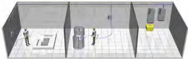
Figure 2. Centralised chemical dosing, application and rinsing system that keeps concentrated cleaning chemicals outside of food processing areas.
