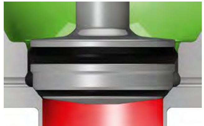
Figure 2a. Seat seal arrangement: radial top – axial bottom (closed).
