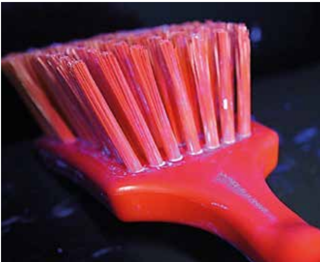
Figure 2a. Drilled and stapled brush after cleaning. UV lotion trapped between the brush block and the bristles.
