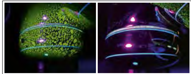
Figure 11. Cleanability test of Detail 4. (Left) Before wipe cleaning, and (right) after wipe cleaning.
