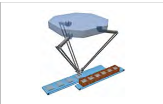
Figure 6. Parallel architecture robots are well known for the high risk of the retention zone (around 2 m 2 ), which houses critical mechanical parts such as motors and oils directly above the product.
