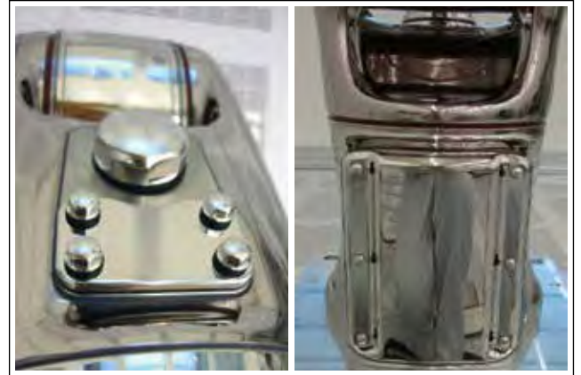
Figure 7. Hygienic design of screw connections. (Left) Hygienically designed screws, and (right) installation lid.
