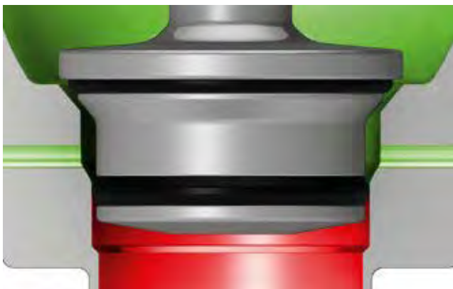
Figure 3b. Seat seal arrangement: axial top – radial bottom (open).
