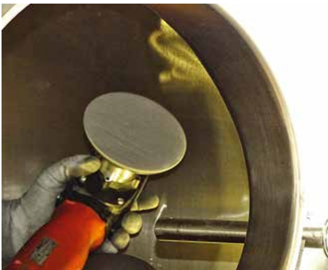
Figure 4. Local refurbishment of scratches by mechanical grinding.
