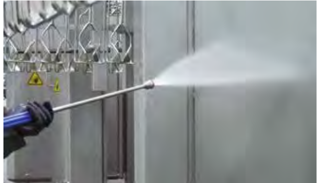
Figure 2. Spraying of a water flat fan onto a surface.
