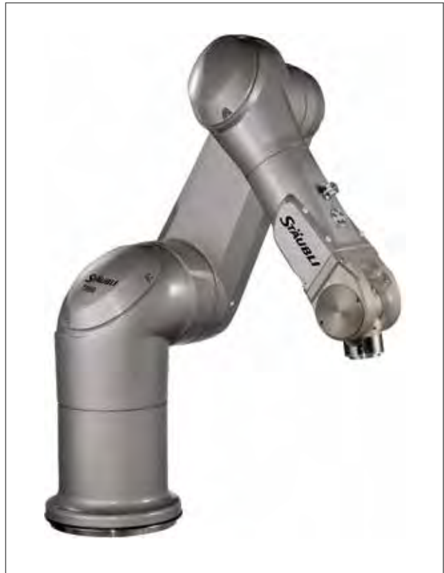
Figure 10. The 6-axis robot co-developed with ECOLAB for compatibility with detergent and sterilising solutions, including foam.
