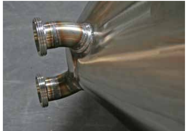
Figure 1. A stainless steel component that shows the typical welding discolourations, imperfections, impurities and contamination generated during fabrication.
