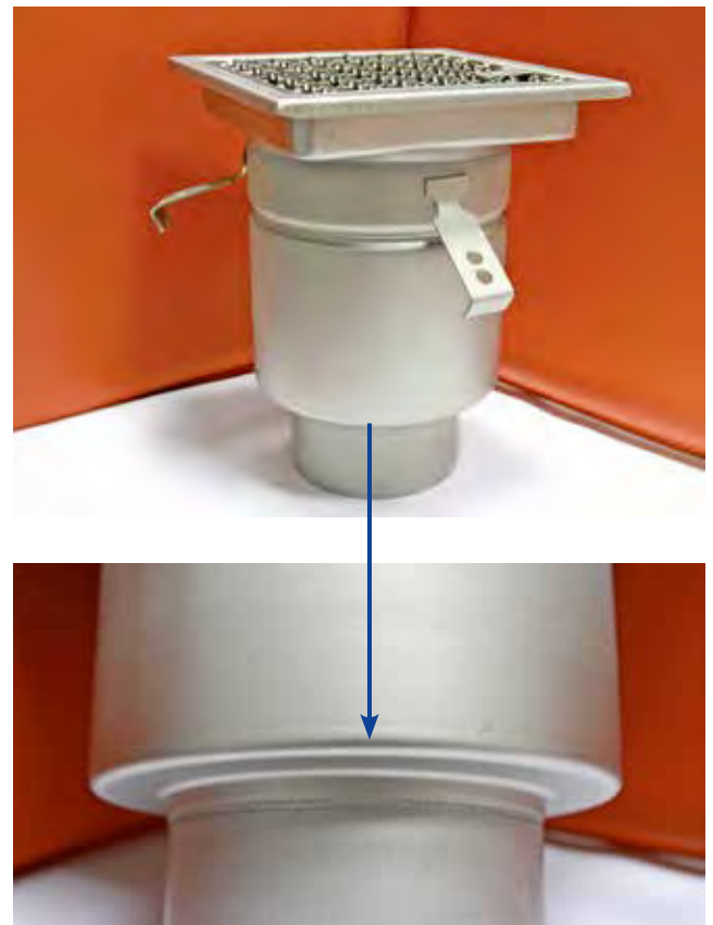
Figure 1. Pressed body. The arrow points to the smooth bottom surface of a pressed drain body, where absence of welds has eliminated a typical hygiene troublespot.
