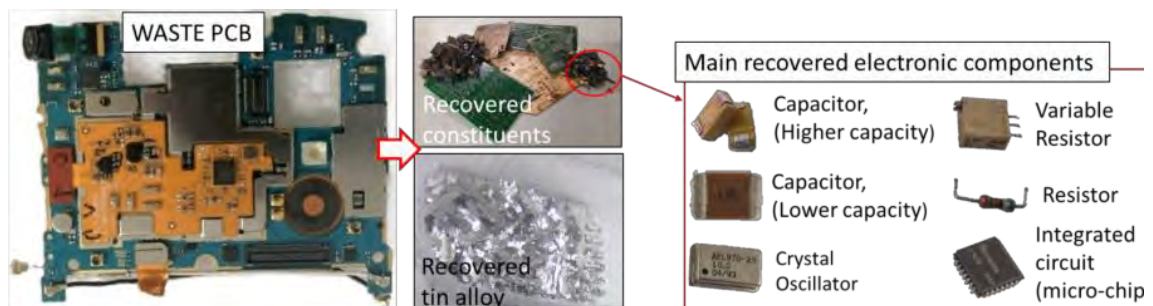
Figure 1. Example of waste PCB and recovered constituents: electric and electronic components, tin alloy and copper layer and fiberglass ply.
