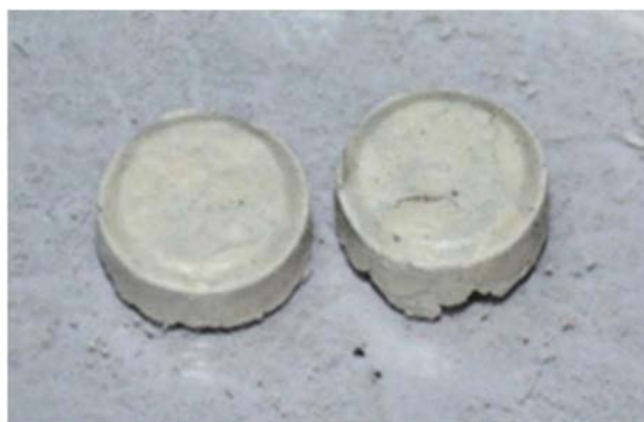
FIG. 4. In house HR-SCMC tablet prepared from IHRs isolated at 40000g.
