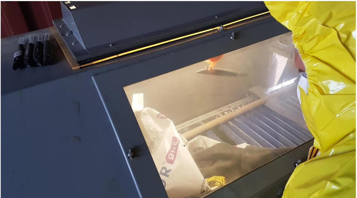
The injections were made per batch, and in the injection plan there are several different concentration batches provided. A typical batch contained 4 m<sup>3</sup> of clean water into which a specified amount of Klozur One was added. From the mixing unit, the proper solution of Klozur One is transferred into the injection tank.
