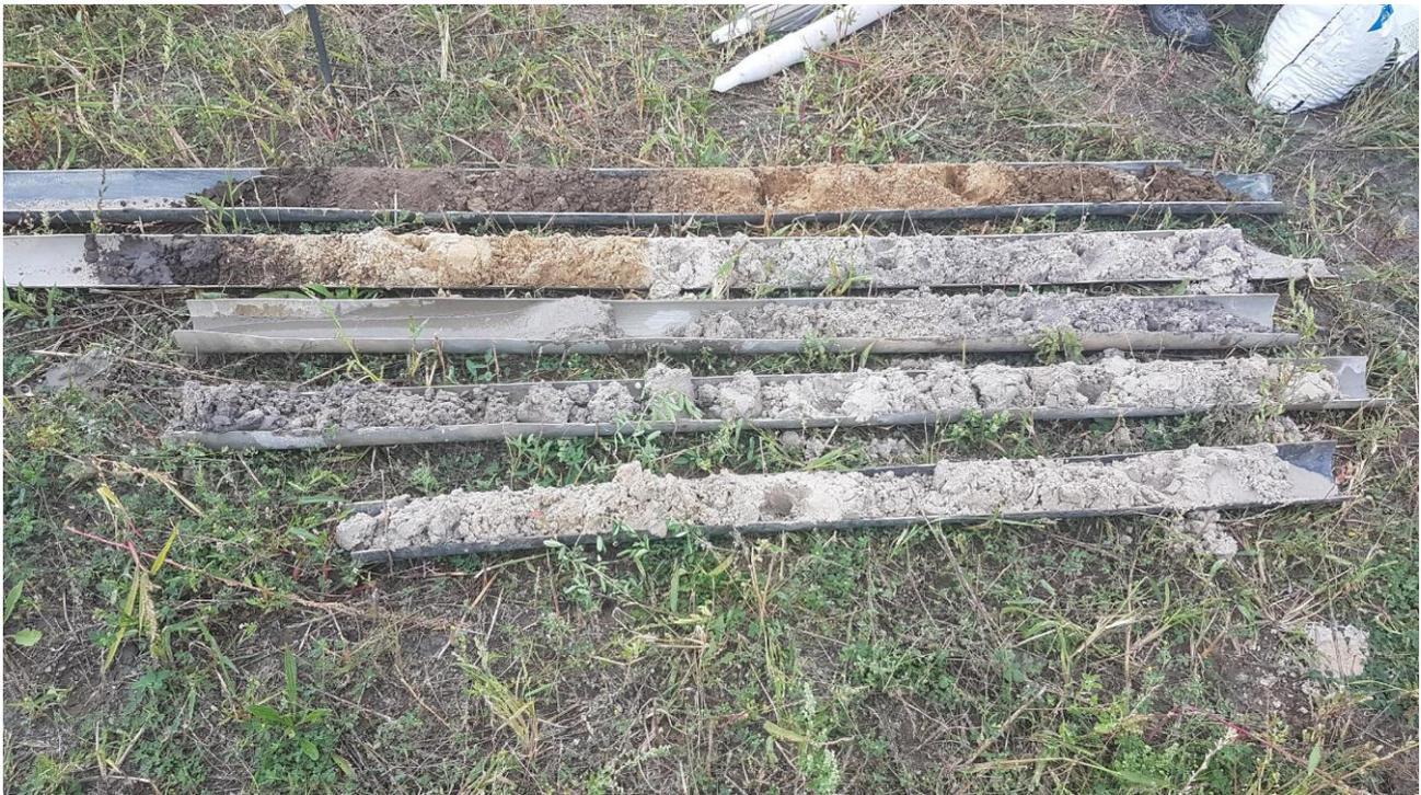
Drill core borehole (sonic drill)
