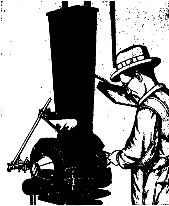
FIG. 28.—Multiple guarding of grinding wheels. (Courtesy of the Surty Manufacturing Company, Inc.)
