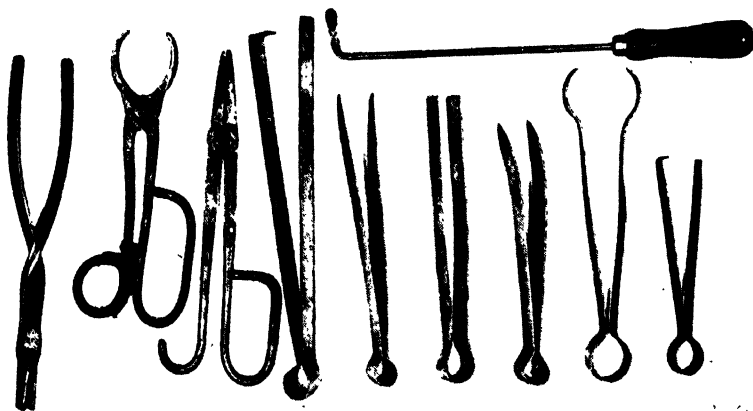
FIG. 80.—An assortment of hand tools for press work. (Courtesy of the Ford Motor Company.)
