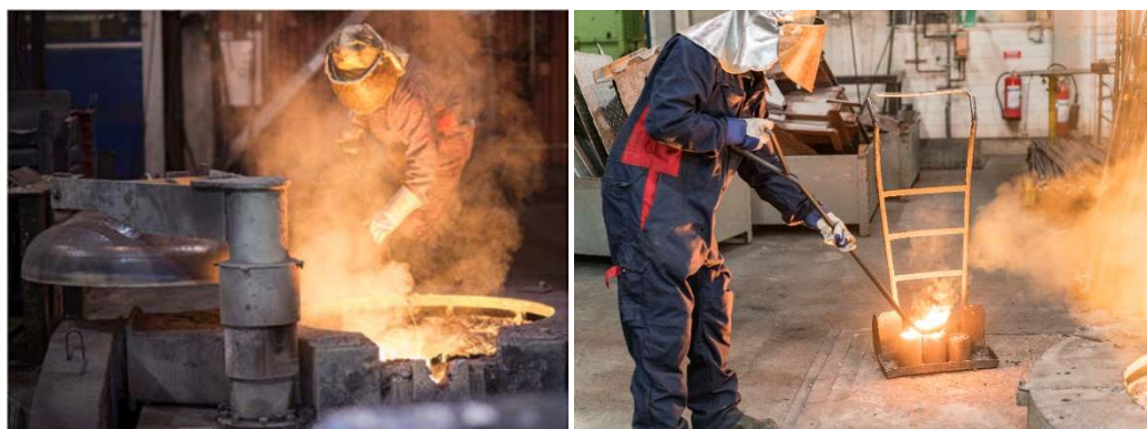
FIG. 8. Sampling of the melting batch.
