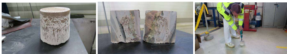
FIG. 2. View of SIAL final product and its compressive strength test (under hot water application).
