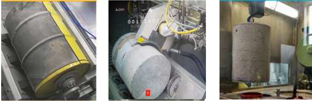
FIG. 4. Left: dismantling of a drum after cutting in the FZA; middle: milling; right: homogeneously cemented waste matrix after milling.
