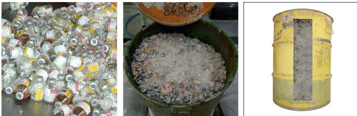
FIG. 8. Example of raw waste found inside. glass waste (in some cases in-drum compacted).
