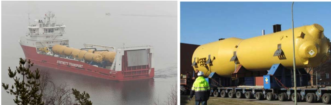
FIG. 11. Arriving vessel with three steam generators (left) and SG outside the treatment hall (right).
