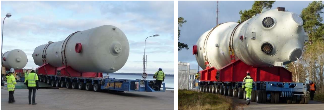
FIG. 1. Steam generator unloaded from sea going vessel (left) and transported to the buffer storage (right).
