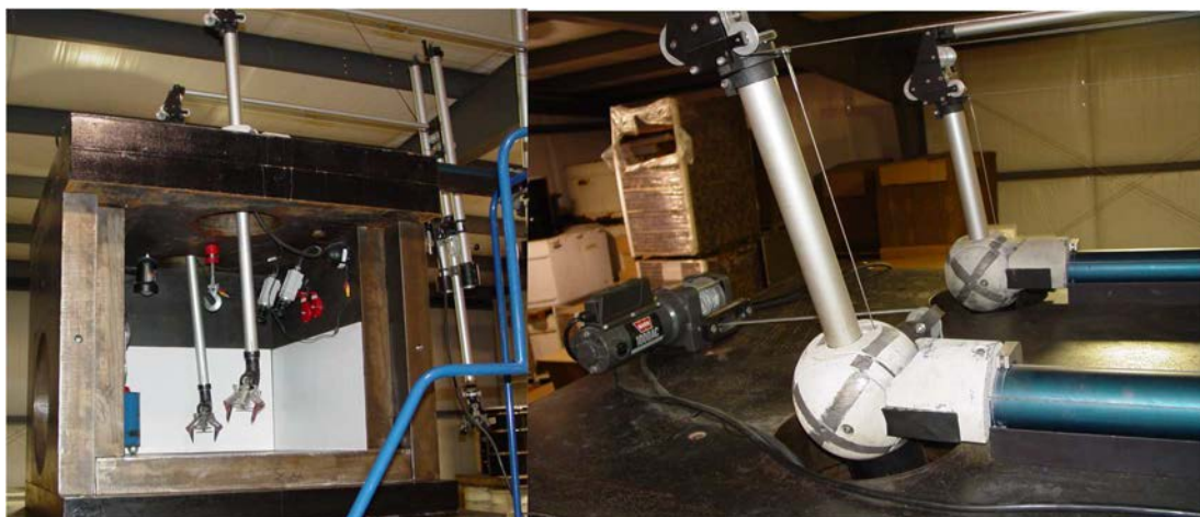
FIG. 3. Contractor's mobile hot cell.
