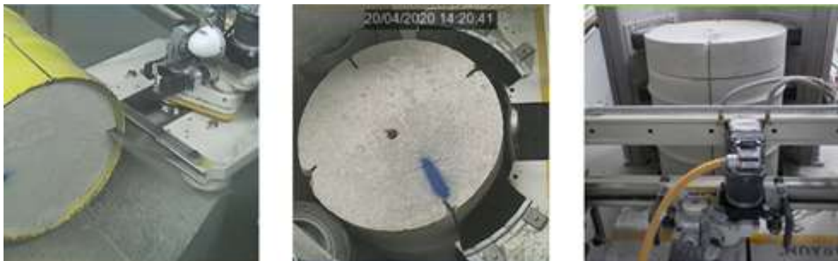
FIG. 5. Dismantling of a in-homogenous waste drum with the cutting tool of the FZA
