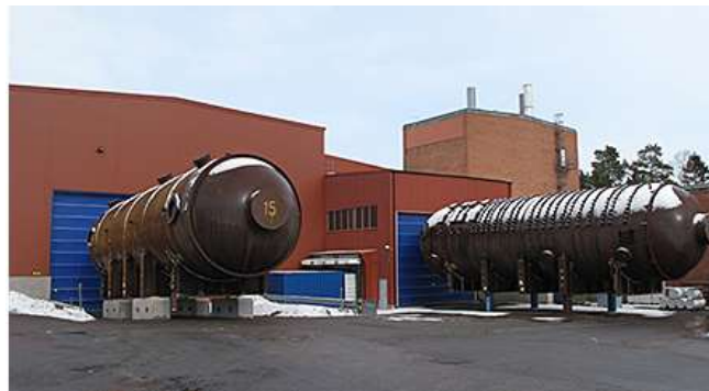
FIG. 2. Boilers awaiting treatment outside Cyclife metal treatment facility.
