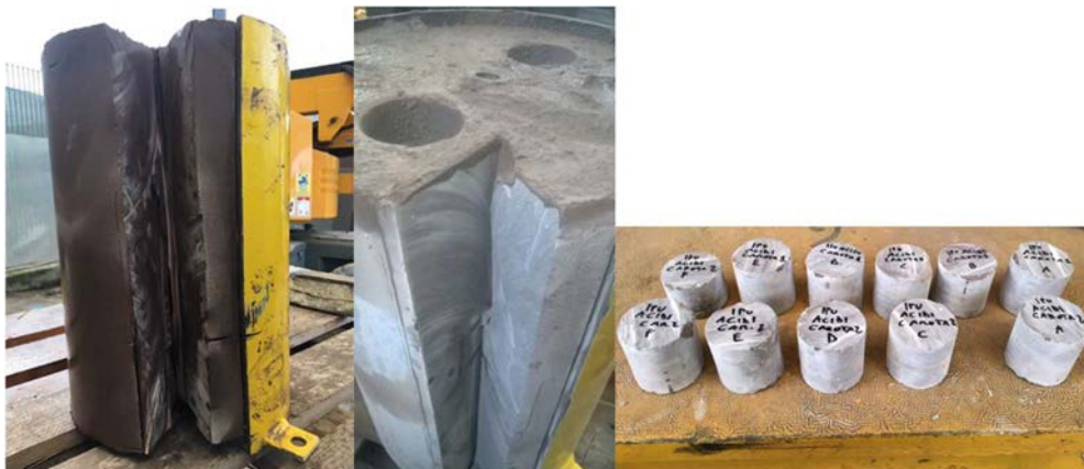
FIG. 3. Drum sectioning and coring.
