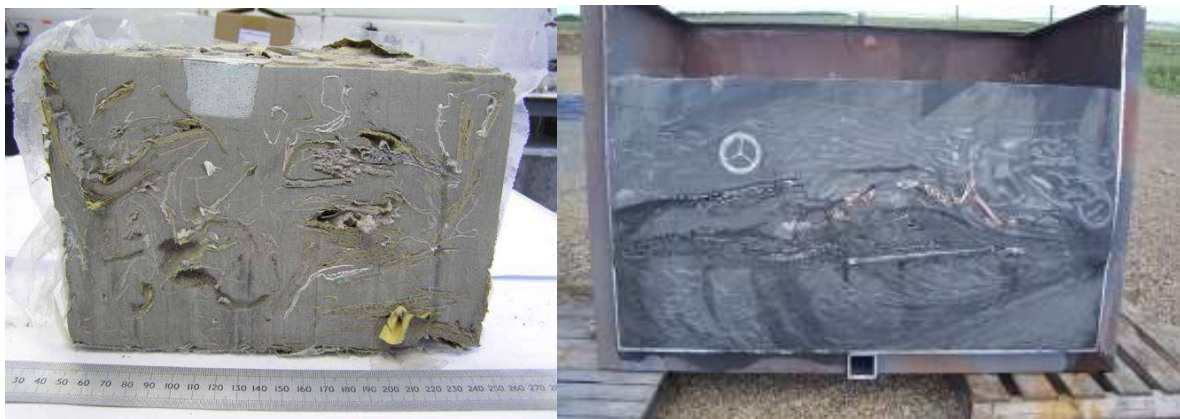
FIG. 4. Cross section observation of final solid product after pouring application.
