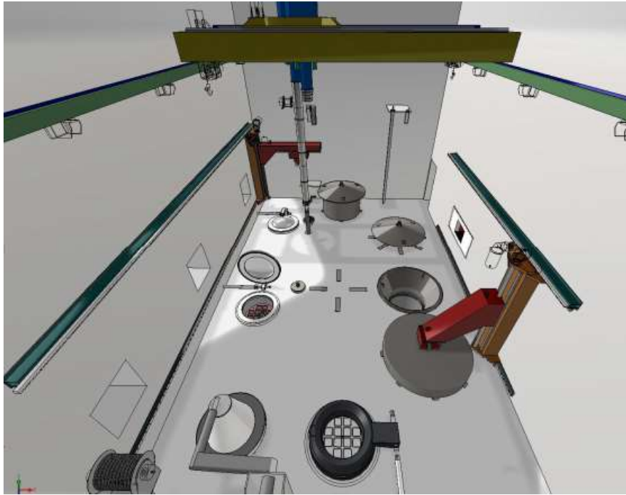
FIG. 7. Fuel handling cell in the encapsulation plant. Courtesy Posiva Oy [1].
