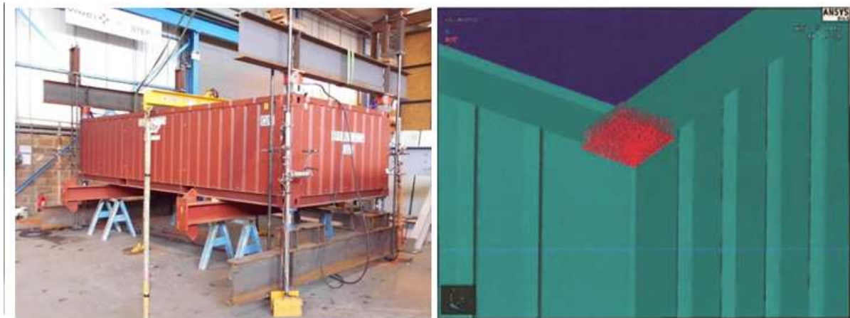
FIG. 3. Container testing and associated FEA model.
