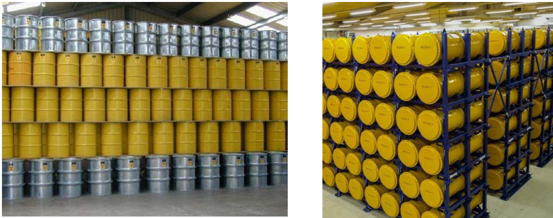
FIG. 2. Left: old storage concept of tightly stacked drums [1]; Right: new storage concept.
