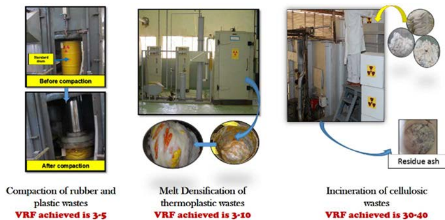
FIG. 1. Volume reduction techniques for combustible O&M wastes (VLLW and LLW).
