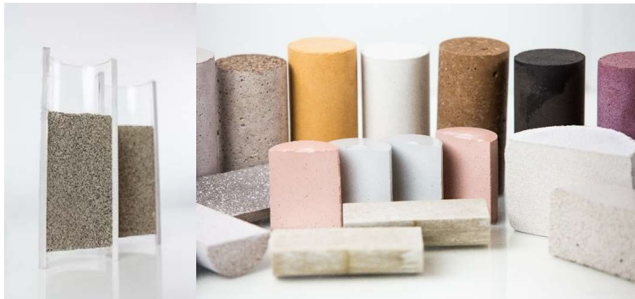
FIG. 3. Cross section observation for series of SIAL samples solidified with different waste streams (resin, sorbents type).
