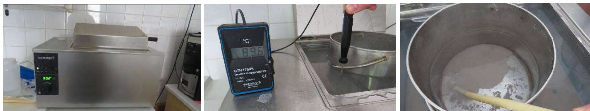
FIG. 1. Pouring application of SIAL under hot water by using water bath set at 90^{\circ}\text{C} .
