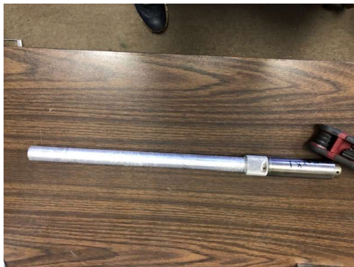
FIG. 2. Example of a JLS Model 6810 source holder.
