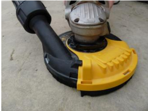
Figure 3 Grinder with on-tool extraction (Source HSE, GB)
