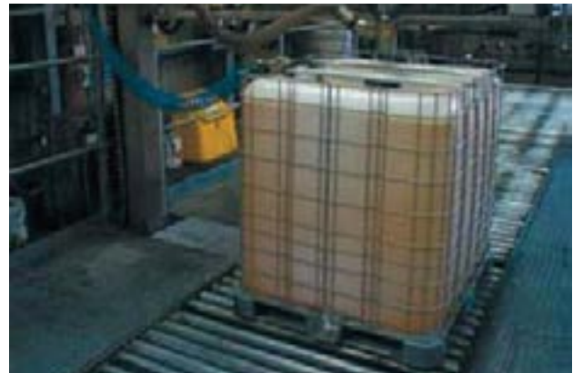
Figure 4. Typical plastic IBC
