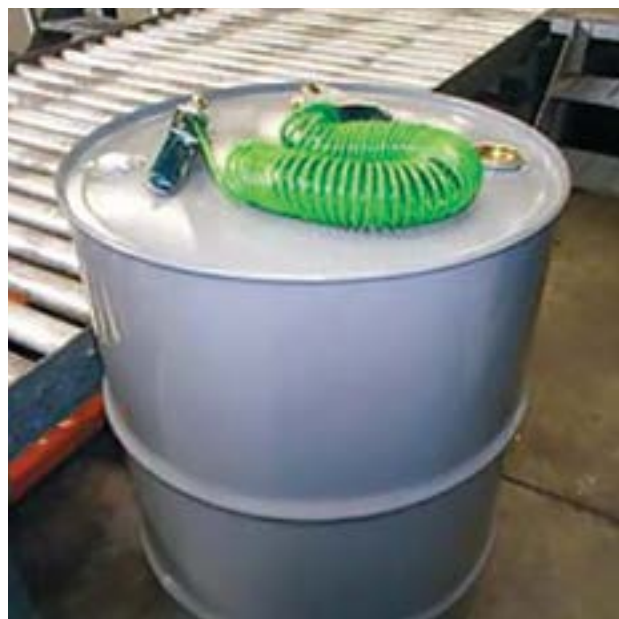
Figure 5. Typical mobile earthing for drums
