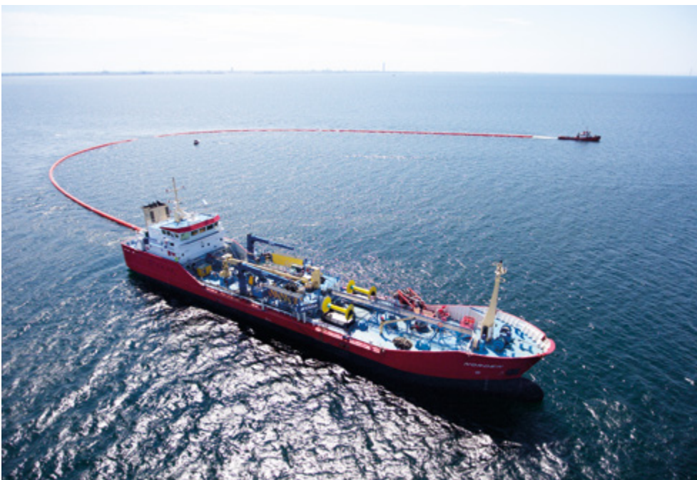
Stand-by Oil Spill Response Vessel Norden during a drill with oil boom deployment.
