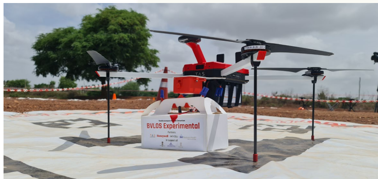
Figure 2: A MEDcopter X4 drone in Beyond Line of Sight (BVLOS) operations in India ( MEDcopter X4 , by Nambi2015, Wikimedia Commons, licenced under CC-BY 4.0 )
