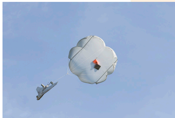
Figure 7: A parachute used to assist the landing of an Eleron-3SV UAV ( Eleron-3SV UAV by Oleg Bor, Wikimedia Commons, licenced under CC-BY 4.0 )
