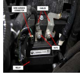
Figure 3 – Intake Air Heater Relay
