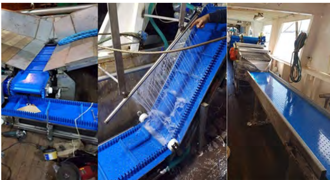
Fig. 15: the figure shows an example of an automation system for sorting and washing the catch
