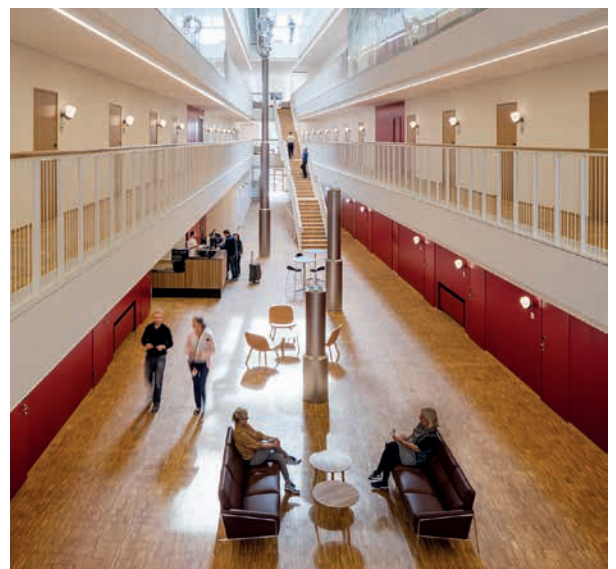
A central indoor open area can provide clear guidance during an evacuation (in an emergency).
