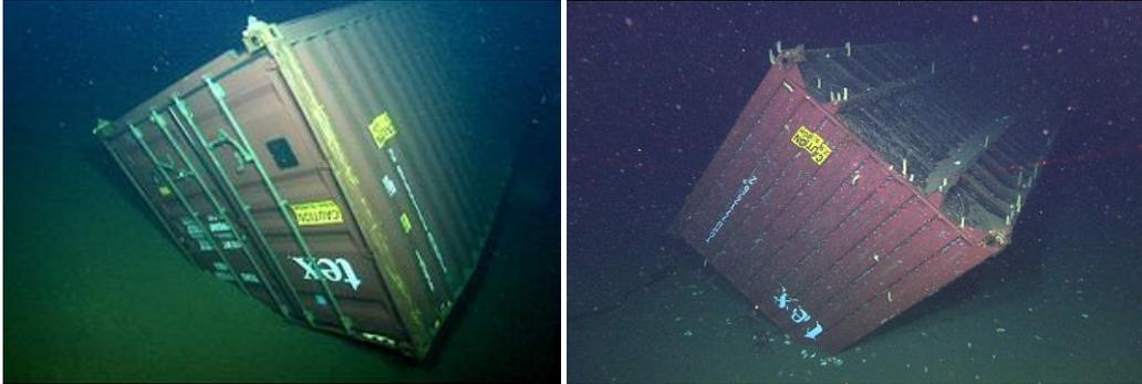
**Figure 17. Container TGHU7712262 in 2004 (left) and 2011 (right). Although colonized by various deep-sea species such as *Neptunea* snails, the container appeared to be in near perfect structural condition. Photo credit: MBARI/MBNMS.**
