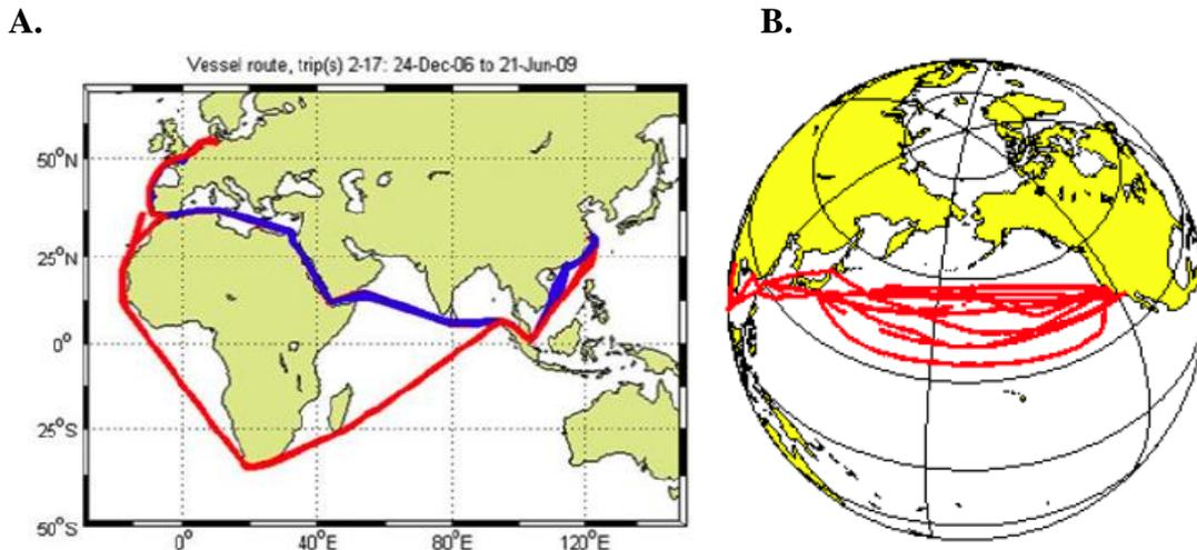
**Figure 20. Compared to a Far East – Europe route (a), the Far East – North America West Coast route of a ship like the *NYK Argus* (b) allows for considerable course alteration and weather avoidance. Red lines in the figure at right show actual routes of the *NYK Argus* over several months. Figures from MARIN 2009.**
