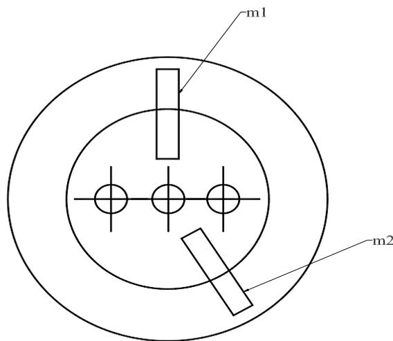
(m1, m2) Macro sections through valve boss/plate welds
