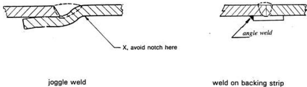
Note : The angle weld can be performed as a "chain-weld"
