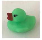
Chemical Environment The blue and green plastic contains an excessive amount of bis(2-ethylhexyl) phthalate (DEHP) and di-isobutyl phthalate (DIBP) (measured values up to 15.0 % and 13.7 % by weight respectively). These phthalates may harm the health of children, causing possible damage to their reproductive system. The solders in the toy contain lead (measured value up to 50.7 % by weight). Lead poses a risk to the environment.
