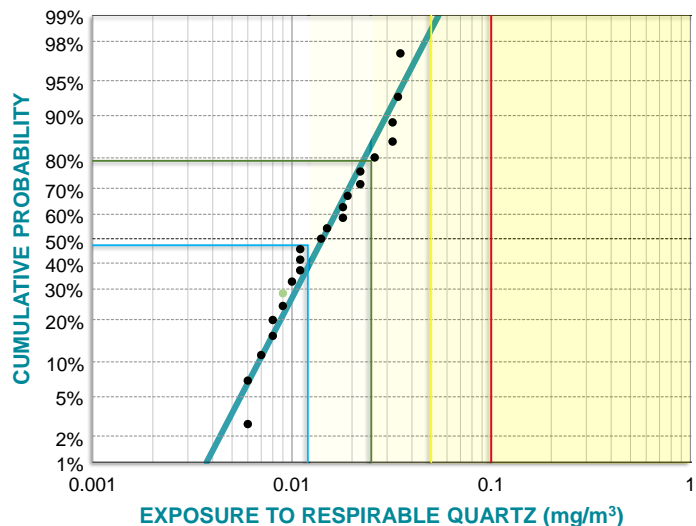
Figure 1.2 Lognormal probability diagram referred to the RCS exposure for the job title C16.04.04 Moulding press operator , working in foundries, constructed from the data set shown in Table 1.4. GM=0.014 mg/m 3 , GSD=1.774, n=23 measurements. The green circle represents a measurement <LOQ.
