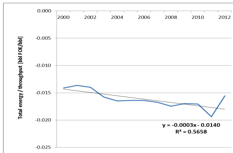
Figure 5.3.7: Difference between average refining energy per throughput (barrels of fuel oil equivalent per barrel of throughput) in Europe and the five competitor regions
