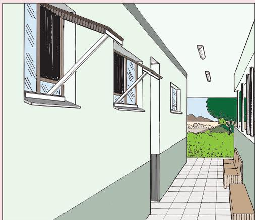
**Situation:** A Swaziland hospital had poor ventilation in a TB ward. The windows could be opened slightly with hooks, but this was insufficient for proper ventilation.
