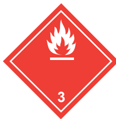
Pictogram for flammable liquid in the UN Model Regulations (Symbol: Flame: black or white; Background: red; Figure 3 in bottom corner; minimum dimensions 100 mm × 100 mm)
