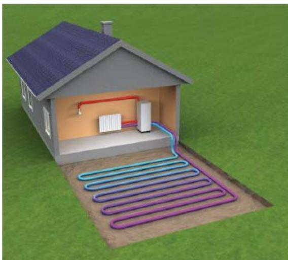
**Image 2.14:** Ground source heat pump for space heating
