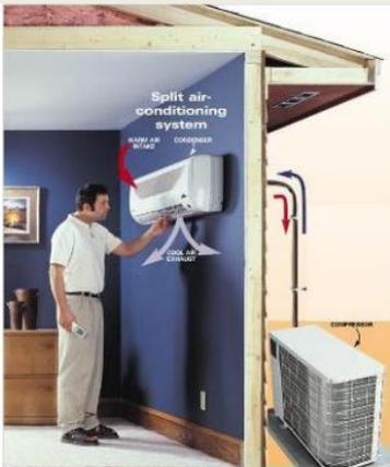
**Image 2.4:** Split air-conditioning: Wall mounted indoor unit and outdoor unit
