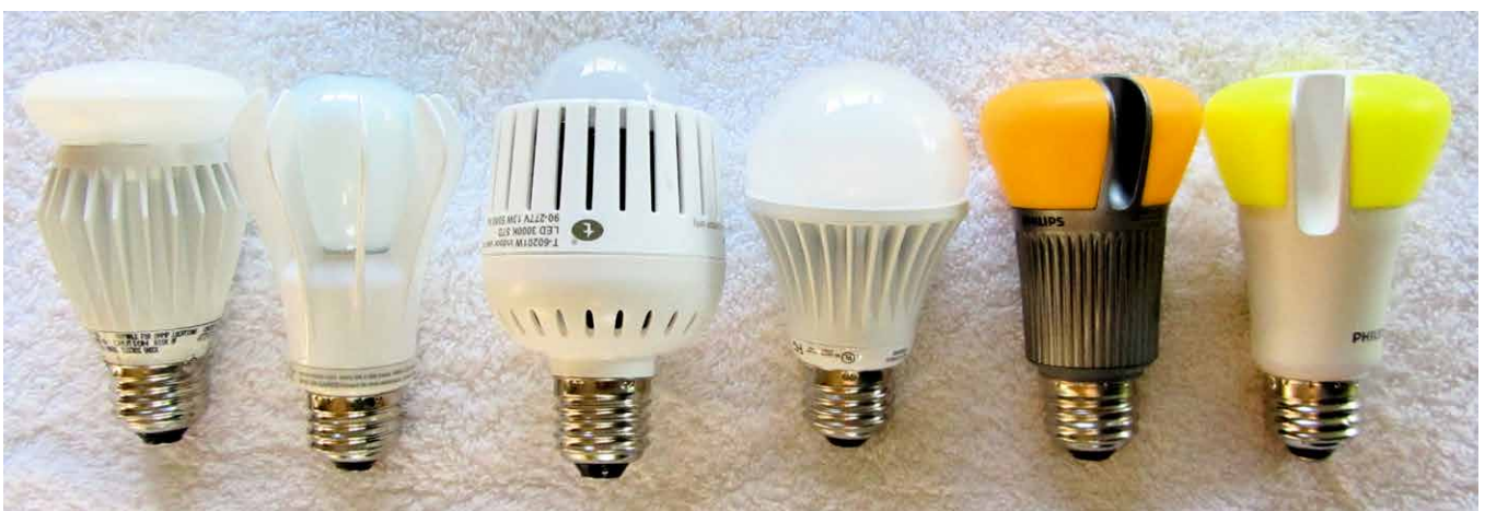
Some of the LED lightbulbs available to the consumer as screw-in replacements for standard incandescent bulbs. Geoffrey A. Landis, 2012. CC BY-SA 3.0 Wikimedia Commons.
