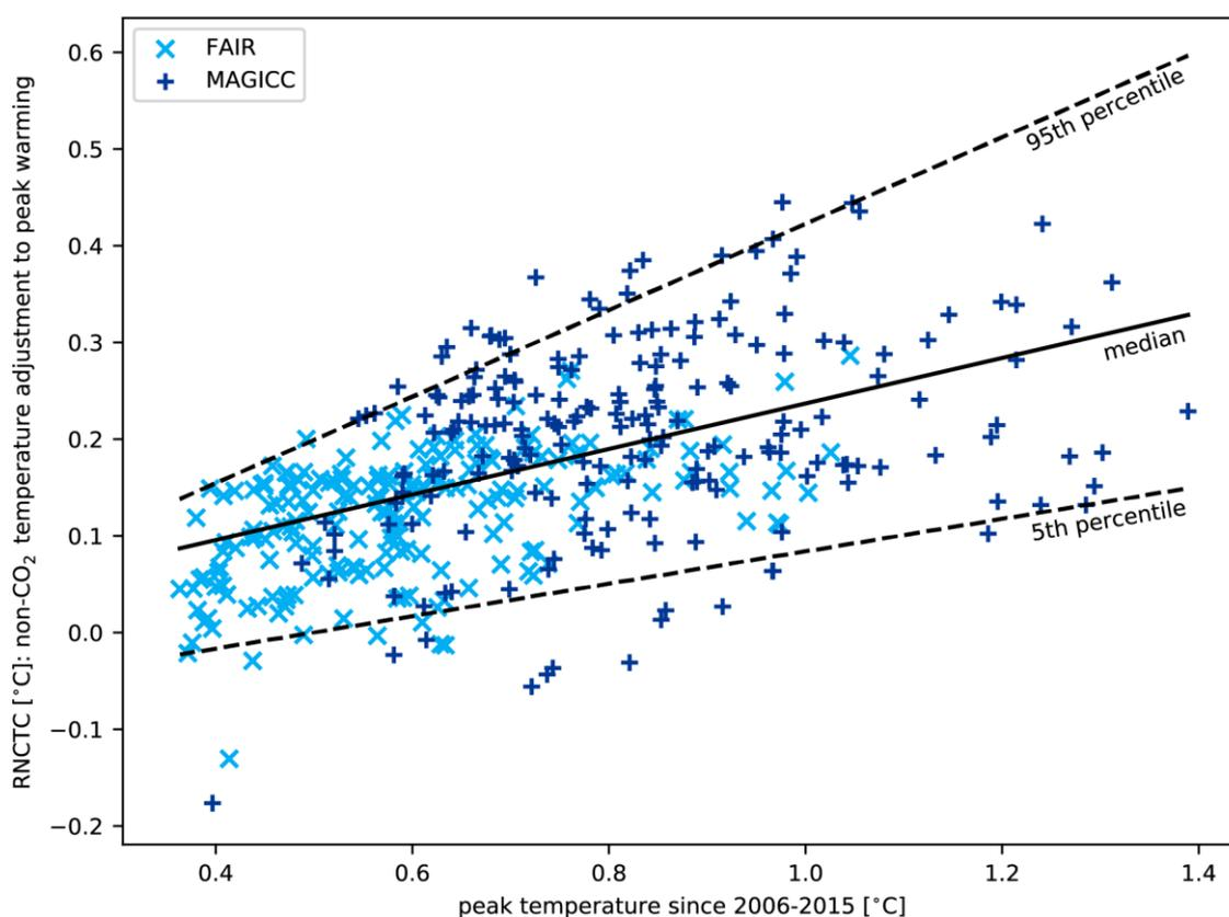
**Figure 2.SM.4:** Relationship of RNCTC with peak temperature in the FAIR and MAGICC models. The black line is the linear regression relationship between peak temperature and RNCTC. The dashed lines show the quantile regressions at the 5th and 95th percentile.
